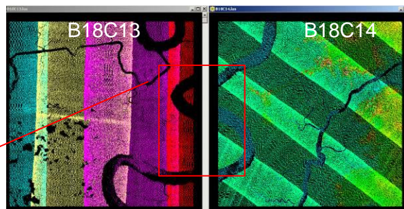
Full point cloud colored by flightline (left) and elevation (right)
