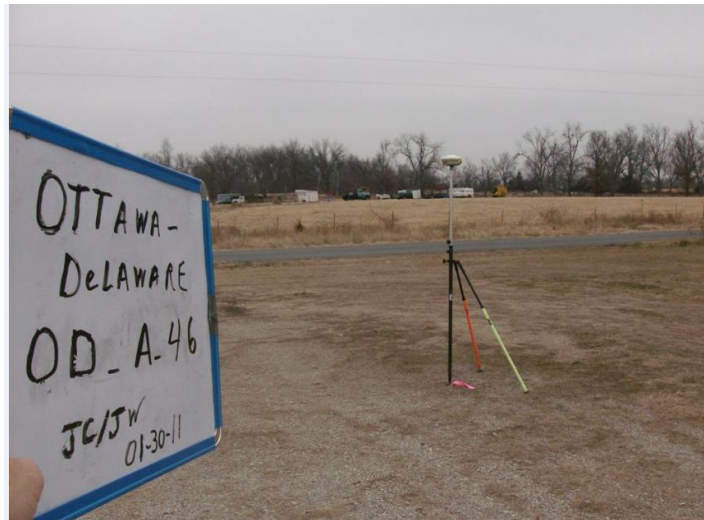
Figure 8: Picture provided for the checkpoint OD_A_46 by the LMSI. Checkpoint is classified to Open Terrain Land Cover Category.
