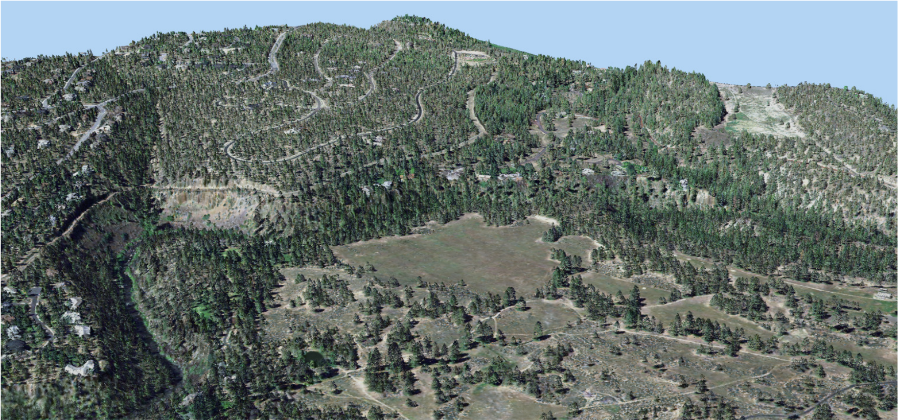
Figure 5.3. View from the east of an area north of Bend, OR along the Deschutes River. Image is a three dimensional LiDAR point cloud with RGB values extracted from a NAIP orthophoto.
