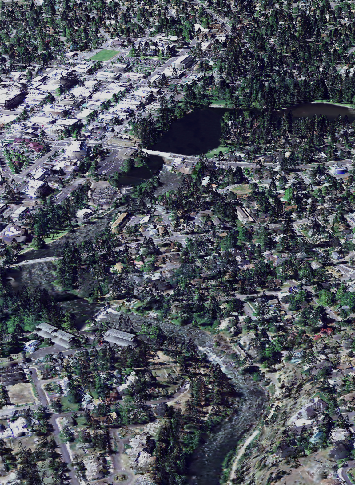
5.3. Oblique view of the Deshutes River in Bend, Oregon. Image is a three dimensional point cloud with RGB values extracted from a NAIP orthophoto.
