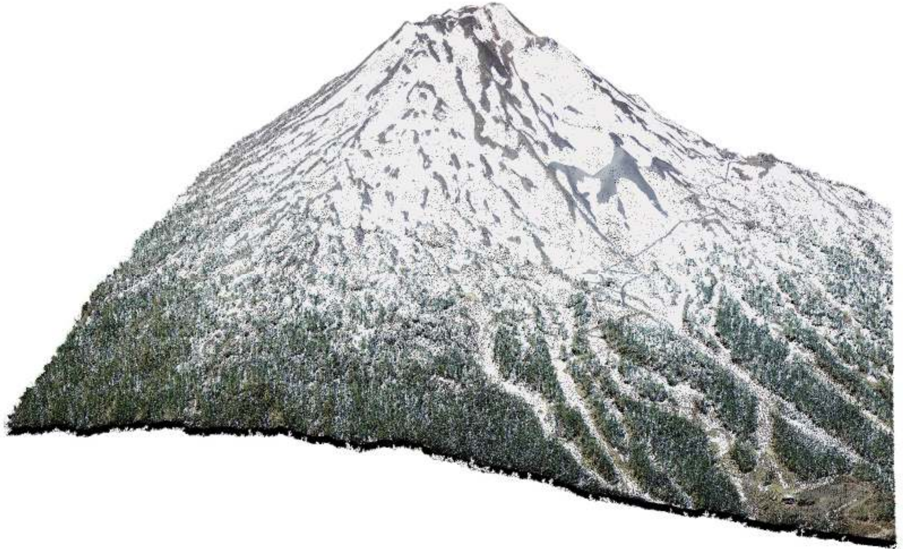
Figure 5.9. Mount Bachelor, west of the city of Bend. Image created from LiDAR point cloud with RGB values extracted from NAIP orthophoto.
