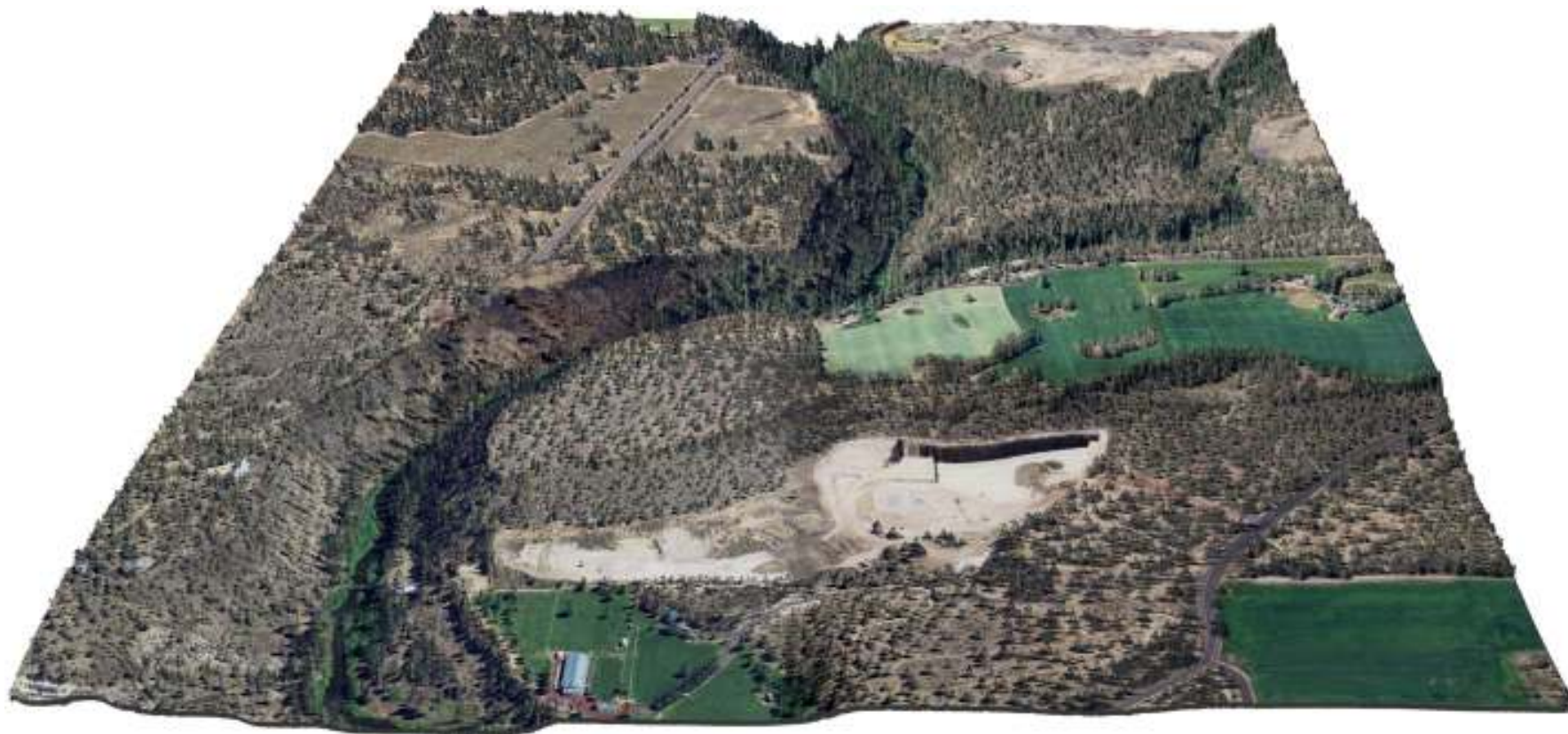
Figure 5.14. Gopher Gulch Airstrip, south of Tumalo State Park, OR. Image created from LiDAR point cloud with RGB values extracted from NAIP orthophoto.
