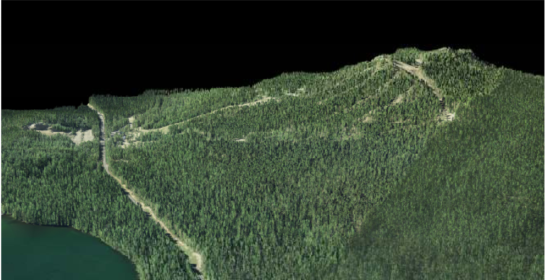
Figure 5.18. Ski hill on Willamette Pass. Image created with a three dimensional LiDAR point cloud with RGB values extracted from NAIP orthophotos.
