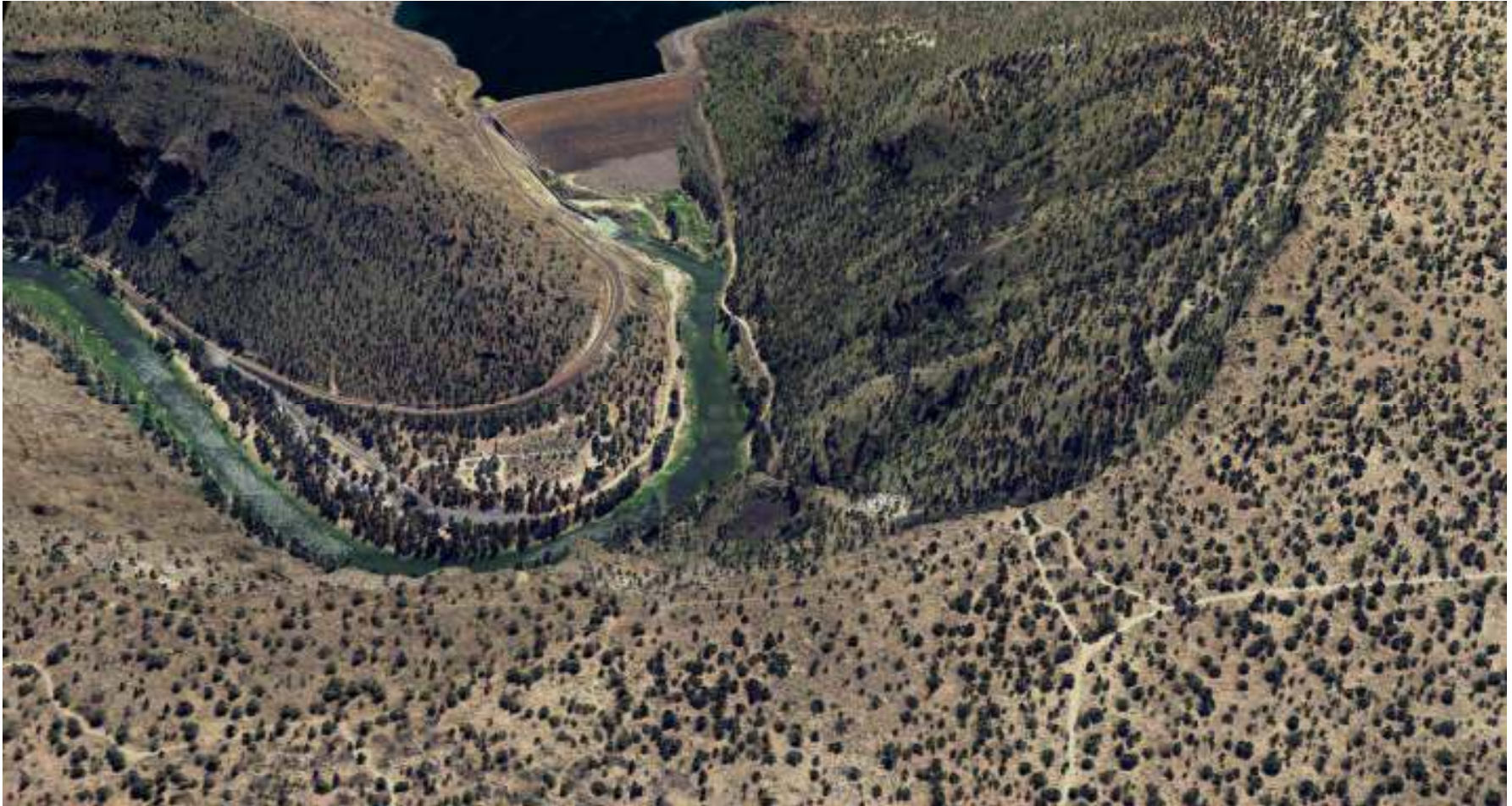
Figure 5.12. The Crooked River below the Bowman Dam and Prineville Reservoir, OR. Image created from LiDAR point cloud with RGB values extracted from NAIP orthophoto.
