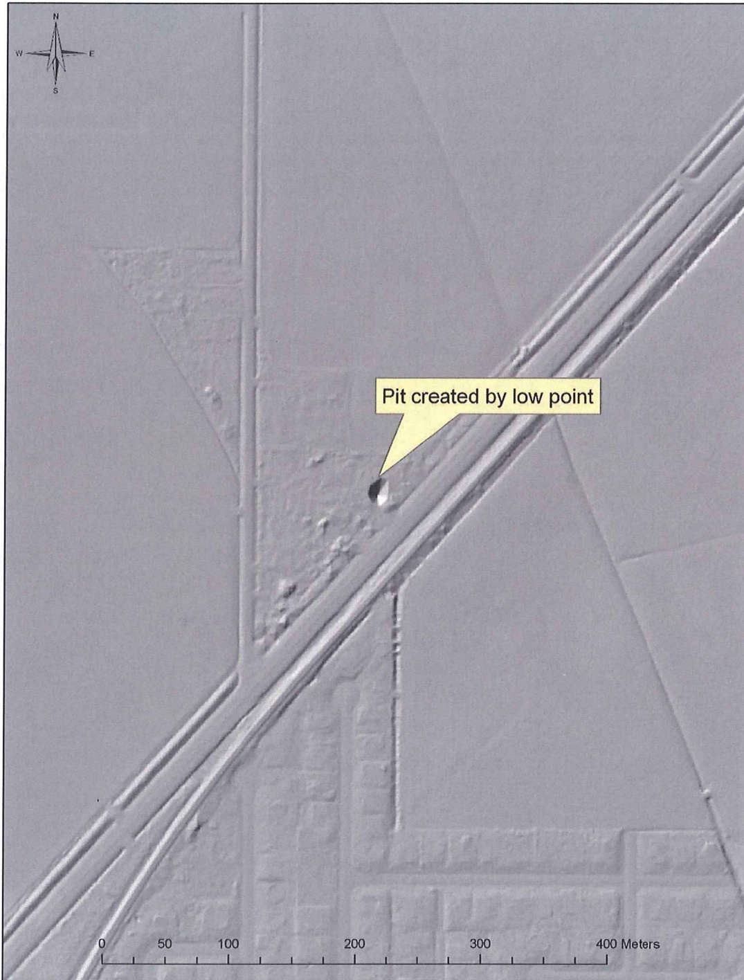
Figure 5. Example of “Pit” caused by low point in ground model. Pits are caused when standing water absorbs the lidar pulse. Pits are evident in ground model as the lowest point elevation is assigned to the grid cell value. Inversely the pit is not observable in the highest hit model as the highest point elevation is assigned to the grid value
