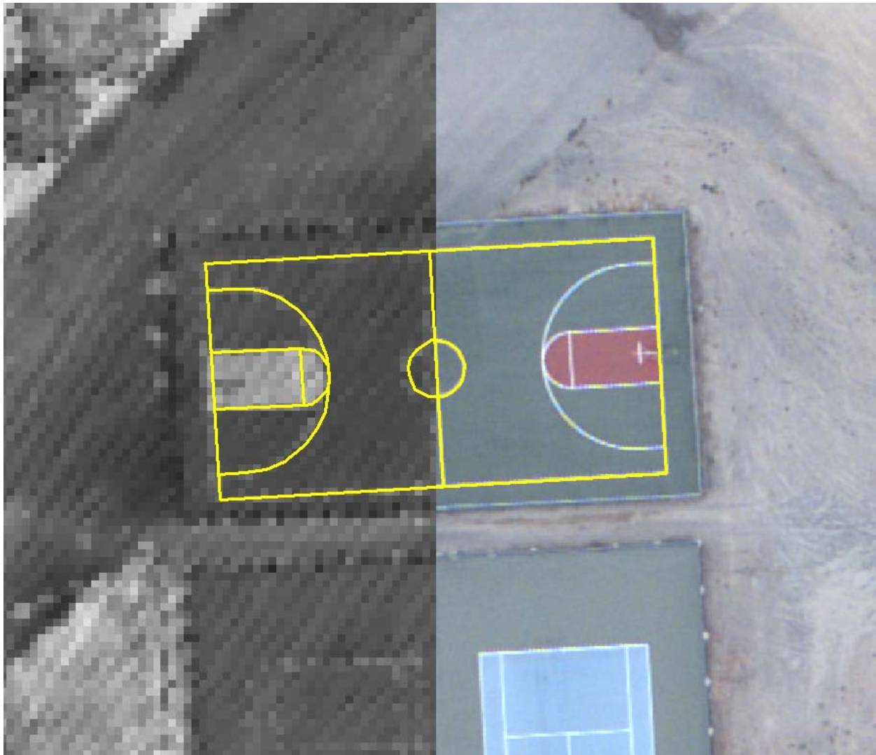
Figure 3. Example of co-registration of color images with LiDAR intensity images
