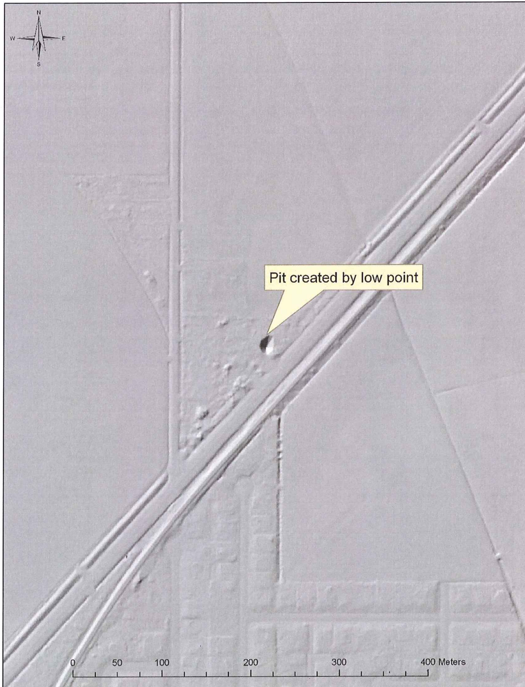
Figure 5. Example of “Pit” caused by low point in ground model. Pits are caused when standing water absorbs the lidar pulse. Pits are evident in ground model as the lowest point elevation is assigned to the grid cell value. Inversely the pit is not observable in the highest hit model as the highest point elevation is assigned to the grid value
