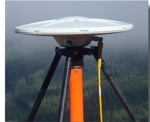
correction to a roving GPS unit. The ground crew uses a roving unit to receive radio-relayed kinematic corrected positions from the base unit. This RTK survey allows precise location measurement ( $\leq 1.5$  cm). **Figure 3.2** shows a subset of these RTK locations.
