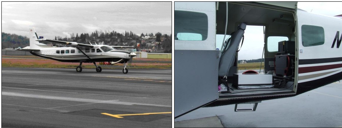
The Cessna Caravan is a powerful, stable platform, which is ideal for the often remote and mountainous terrain found in the Pacific Northwest. The Leica ALS60 sensor head installed in the Caravan is shown on the right.
