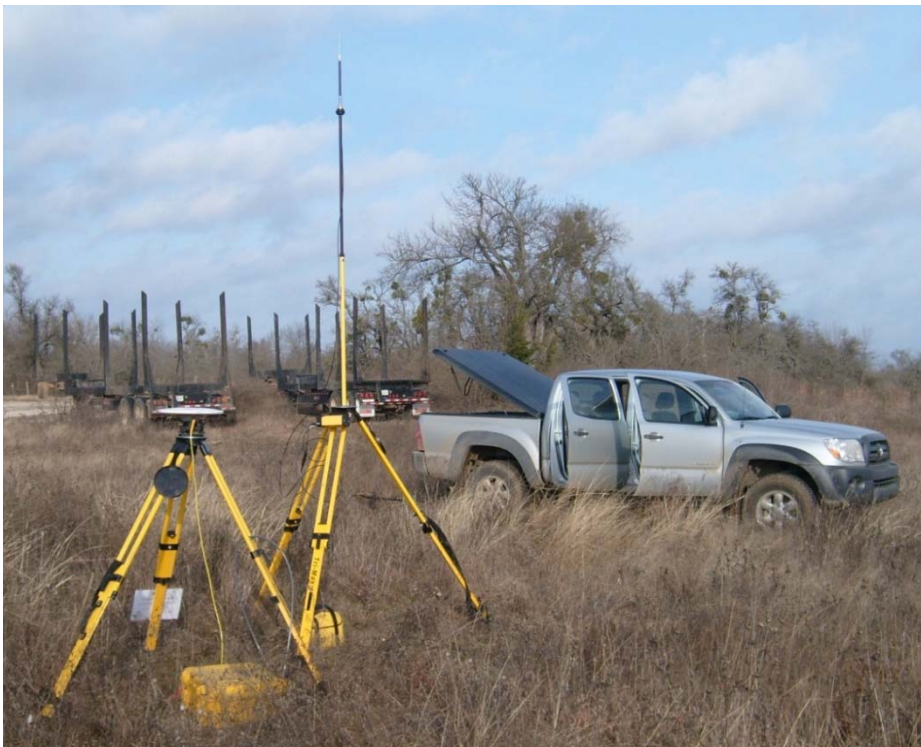
Example of the Trimble GPS survey equipment configured for collecting RTK data.
