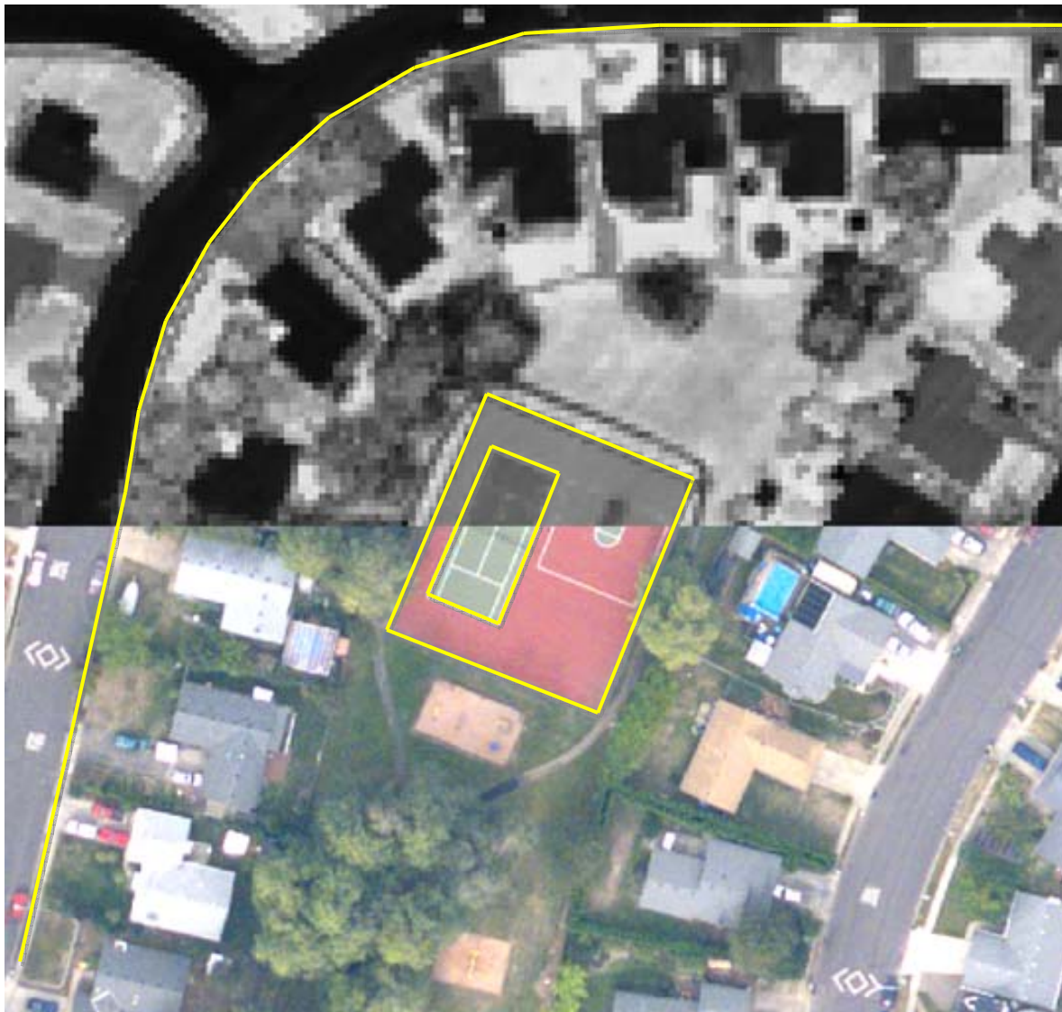
Figure 3. Example of co-registration of color images with LiDAR intensity images
