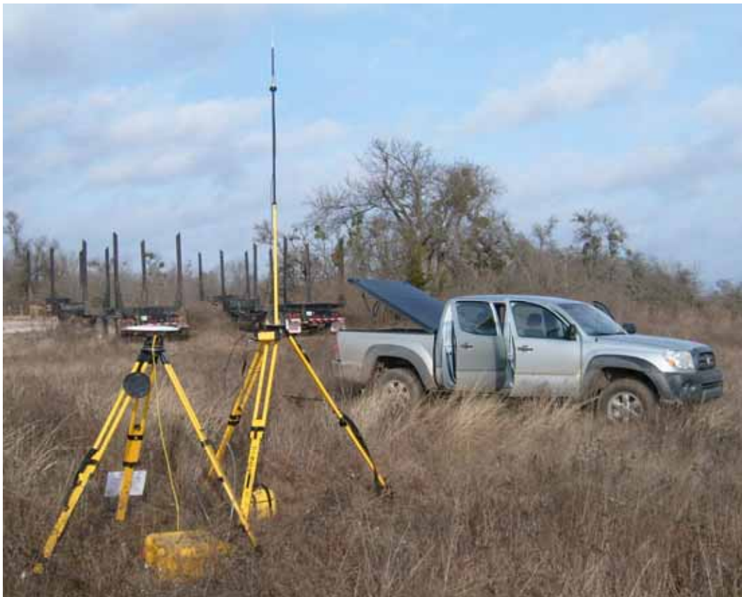
Trimble GPS survey equipment configured for collecting RTK data.
