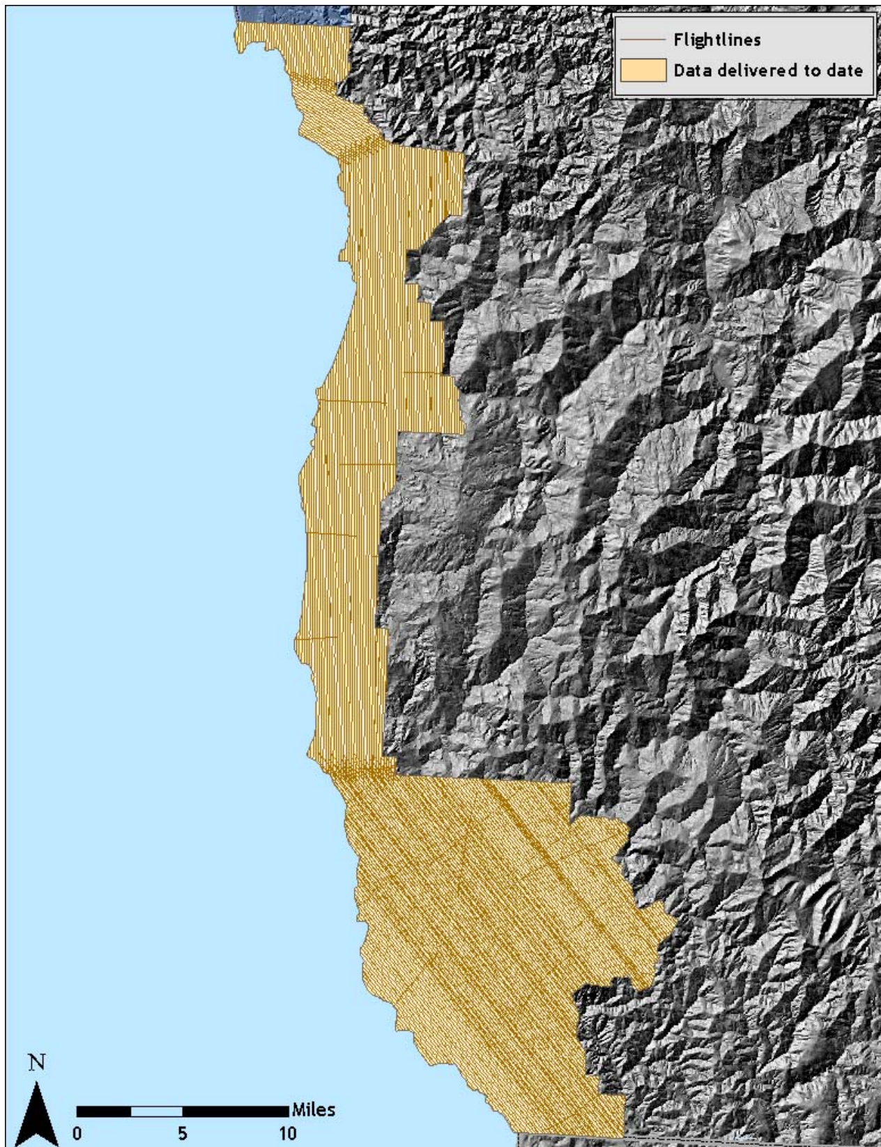
Figure 2.1. Actual flightlines for data delivered to date in the southern Oregon coast study area.
