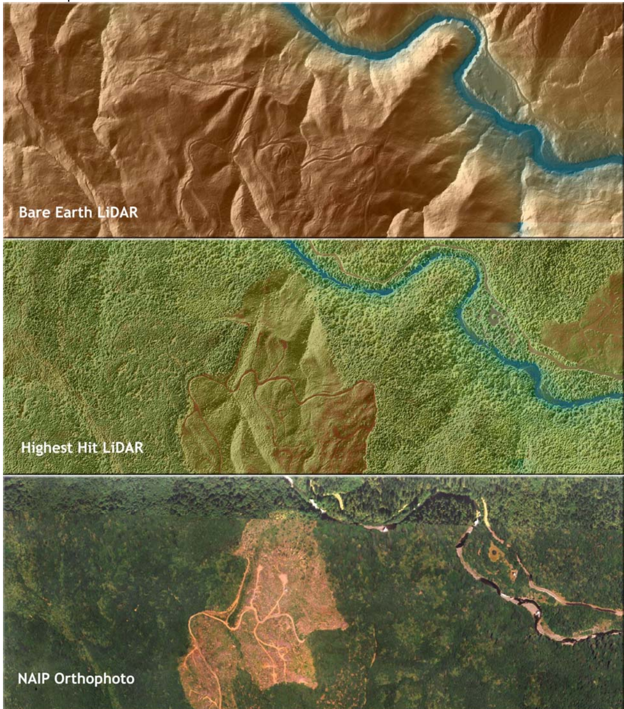
Figure 6.9. View of the confluence of Sixes River and Edson Creek in delivery tile 42124g4. Top image derived from bare earth LiDAR, center image from highest hit LiDAR, and lower image derived from NAIP orthophotos.
