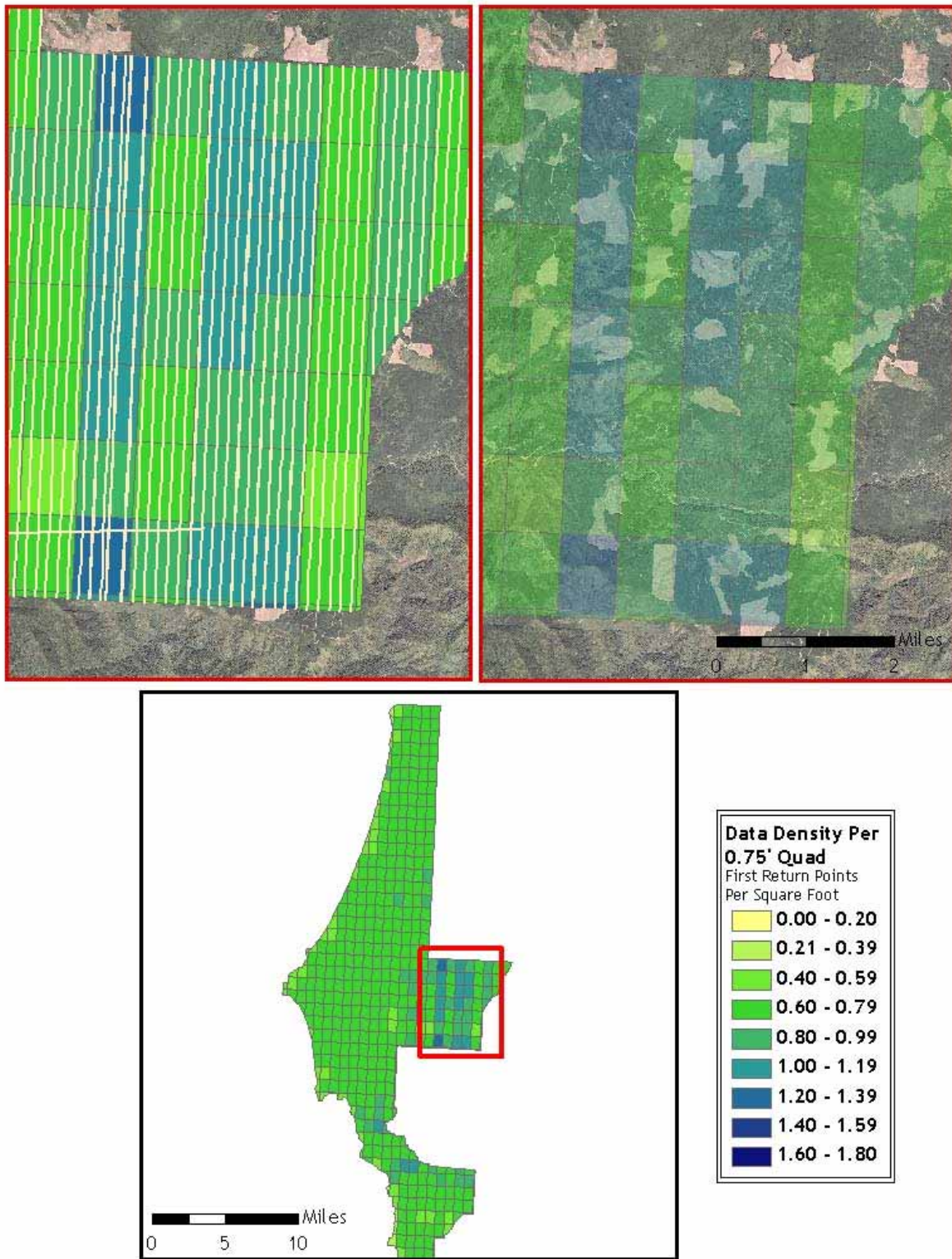
Figure 4.15. Quadrants with higher flightline density result in greater numbers of first return points.
