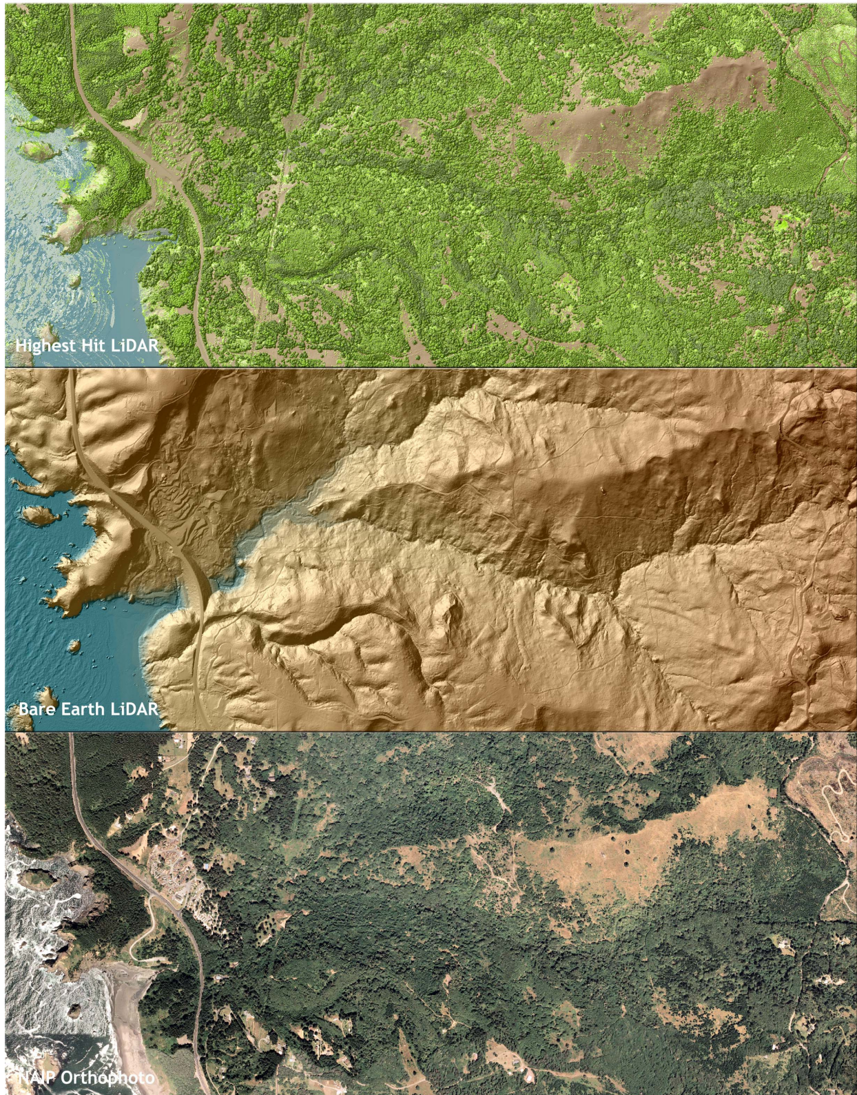
Figure 6.7. Whalehead and Coon Creek at terminus in ocean near Highway 101 (quad42124-b3). Top image derived from highest hit LiDAR, center image from bare earth LiDAR, lower image derived from NAIP orthophotos.
