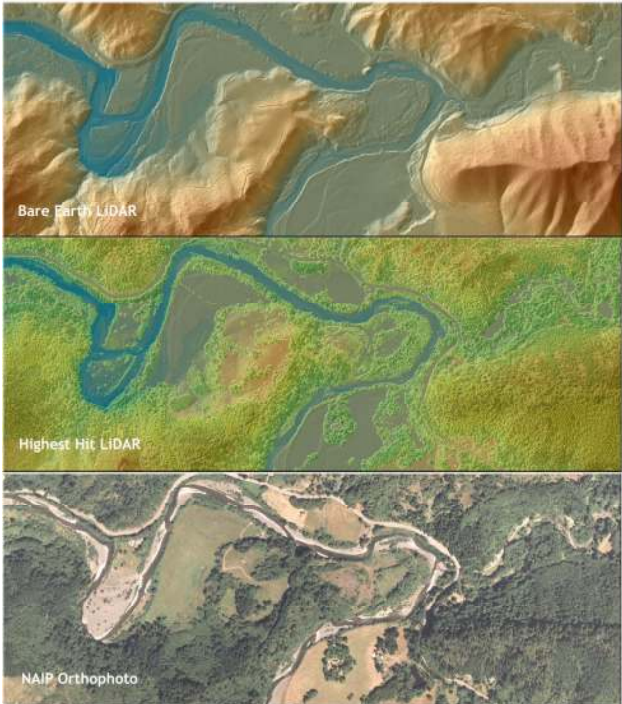
Figure 6.8. View of the Sixes River and Bea Creek confluence in delivery tile 42124g3. Top image derived from bare earth LiDAR, center image from highest hit LiDAR, and lower image derived from NAIP orthophotos.
