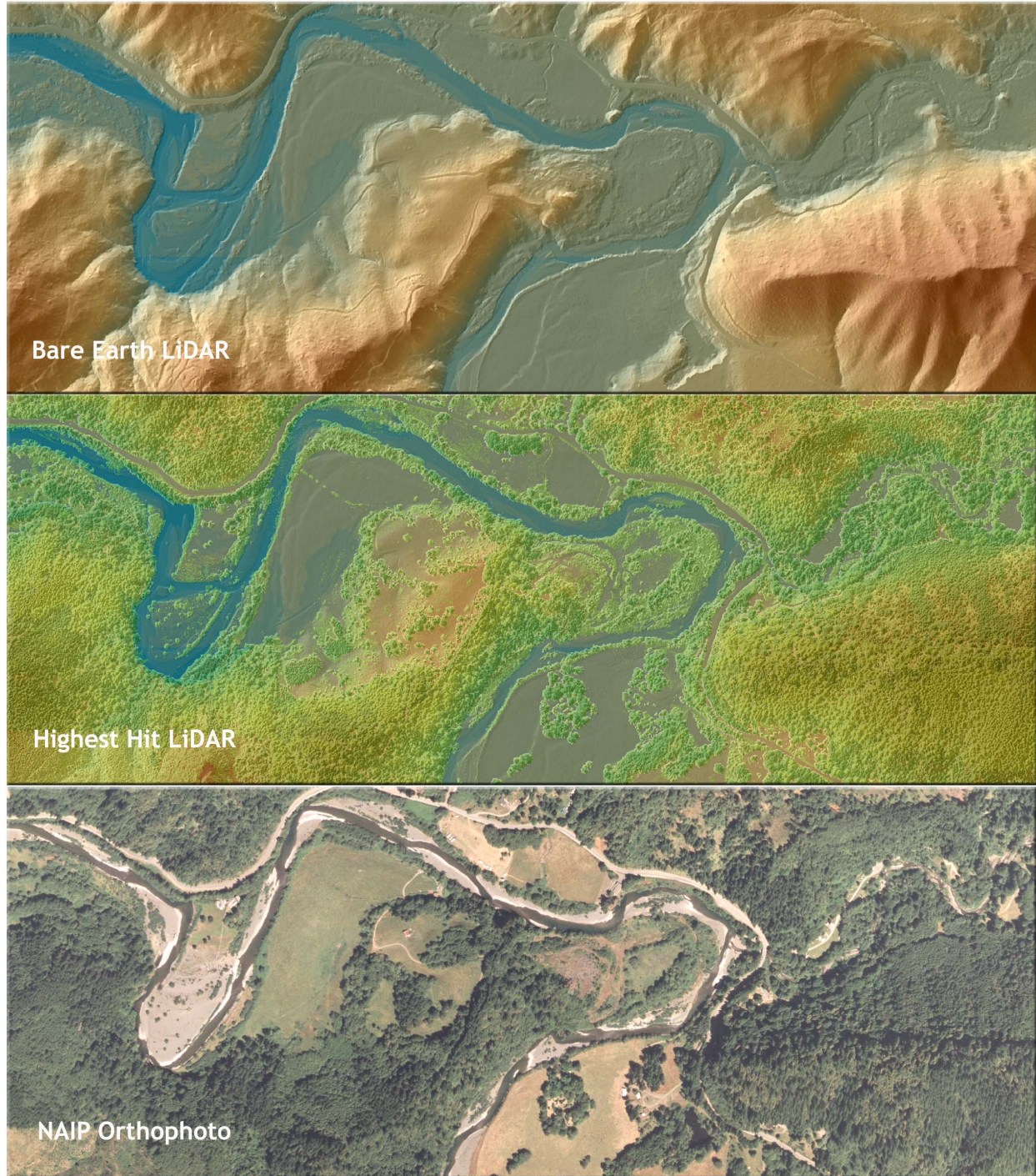
Figure 4.8. View of the Sixes River and Bea Creek confluence in delivery tile 42124g3. Top image derived from bare earth LiDAR, center image from highest hit LiDAR, and lower image derived from NAIP orthophotos.
