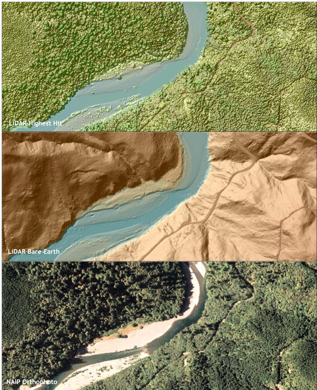
Figure 4.6. Chetco River upstream of confluence with Elk Creek (quad 42124-b2). Upper image derived from highest hit LiDAR, center image derived from bare earth LiDAR, lower image derived from NAIP orthophoto.
