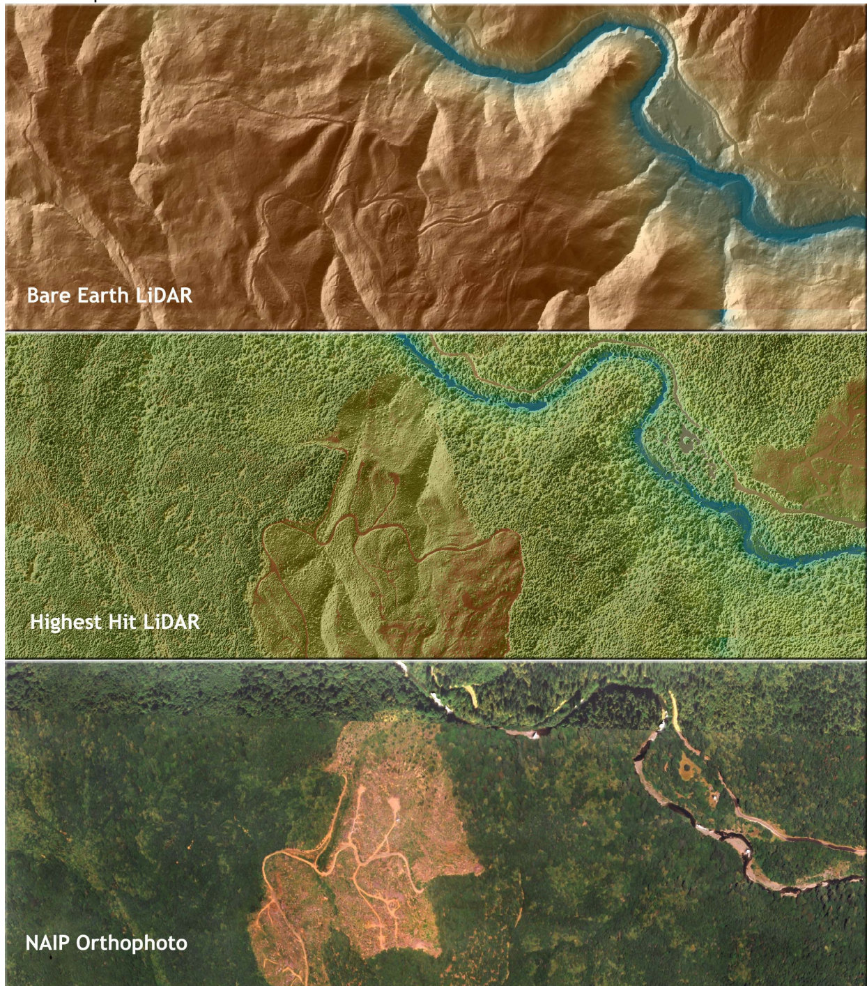
Figure 4.9. View of the confluence of Sixes River and Edson Creek in delivery tile 42124g4. Top image derived from bare earth LiDAR, center image from highest hit LiDAR, and lower image derived from NAIP orthophotos.
