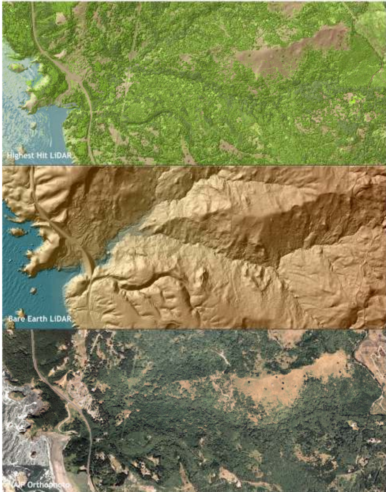
Figure 4.7. Whalehead and Coon Creek at terminus in ocean near Highway 101 (quad42124-b3). Top image derived from highest hit LiDAR, center image from bare earth LiDAR, lower image derived from NAIP orthophotos.
