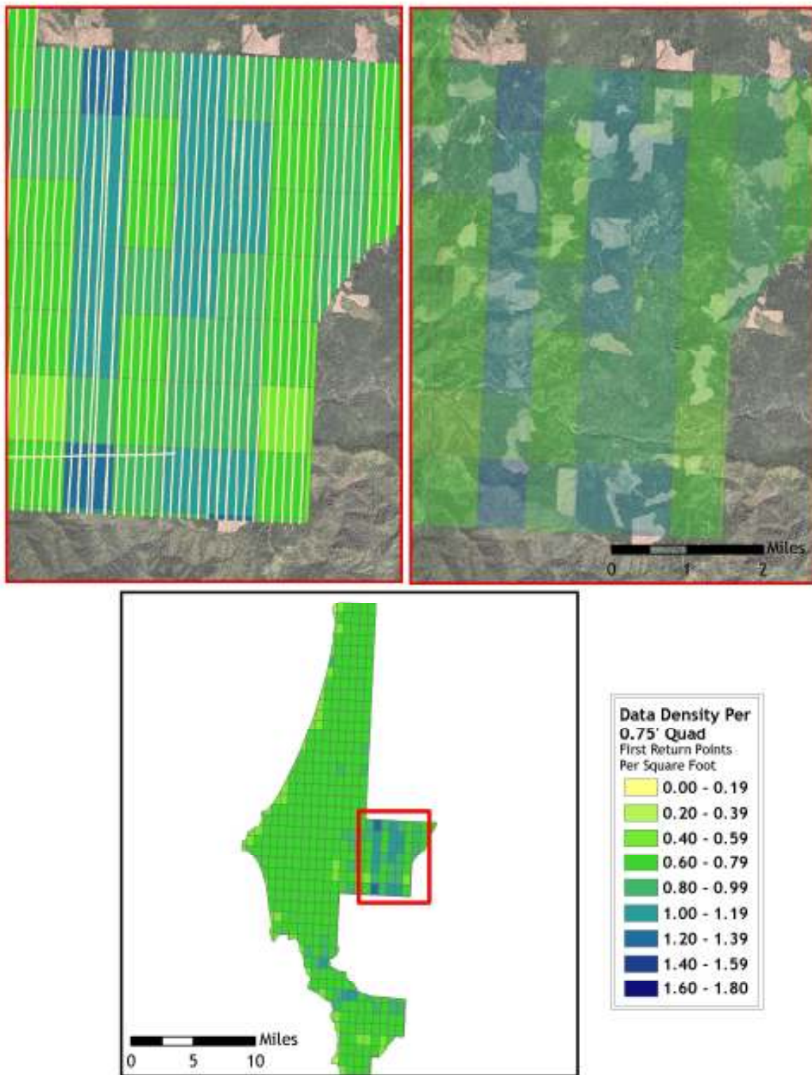
Figure 3.10. Quadrants with higher flightline density result in greater numbers of first return points.
