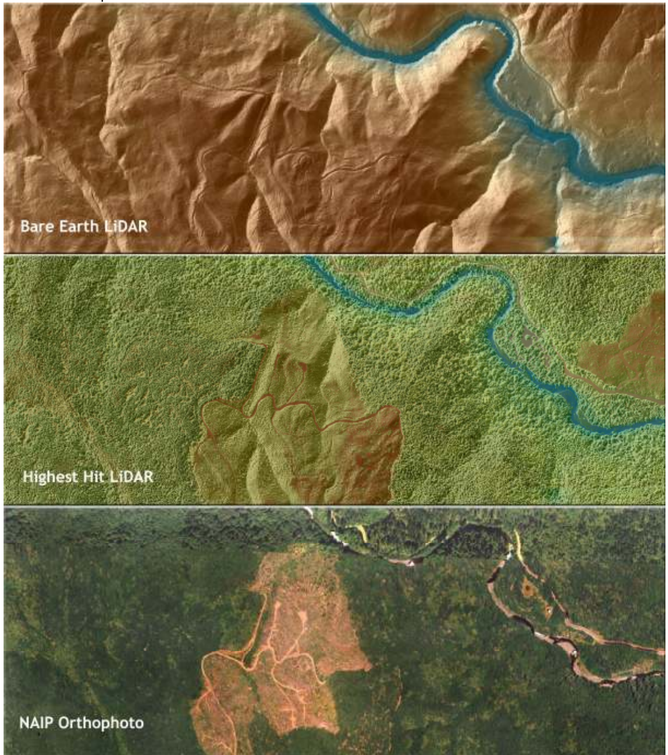
Figure 4.10. View of the confluence of Sixes River and Edson Creek in delivery tile 42124g4. Top image derived from bare earth LiDAR, center image from highest hit LiDAR, and lower image derived from NAIP orthophotos.
