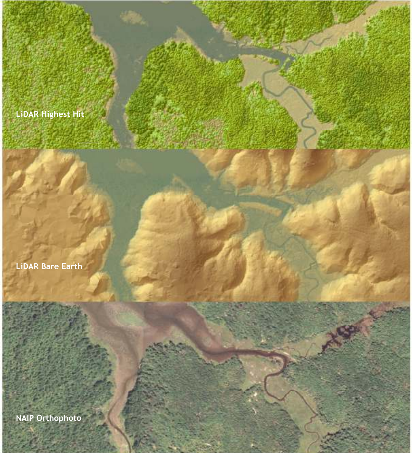
Figure 4.11. Stream confluence entering South Slough just north of Cox Canyon in delivery tile 43124C3. Upper image derived from highest hit LiDAR, center image derived from bare earth LiDAR, lower image derived from NAIP orthophoto.
