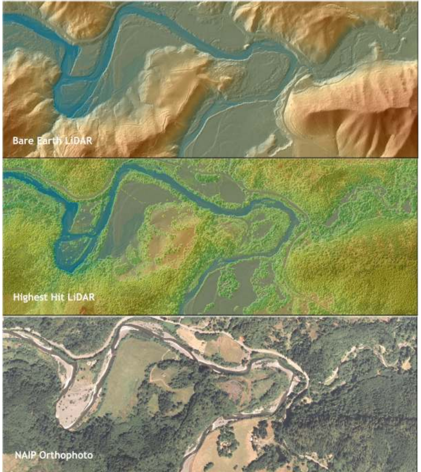
Figure 4.9. View of the Sixes River and Bea Creek confluence in delivery tile 42124g3. Top image derived from bare earth LiDAR, center image from highest hit LiDAR, and lower image derived from NAIP orthophotos.
