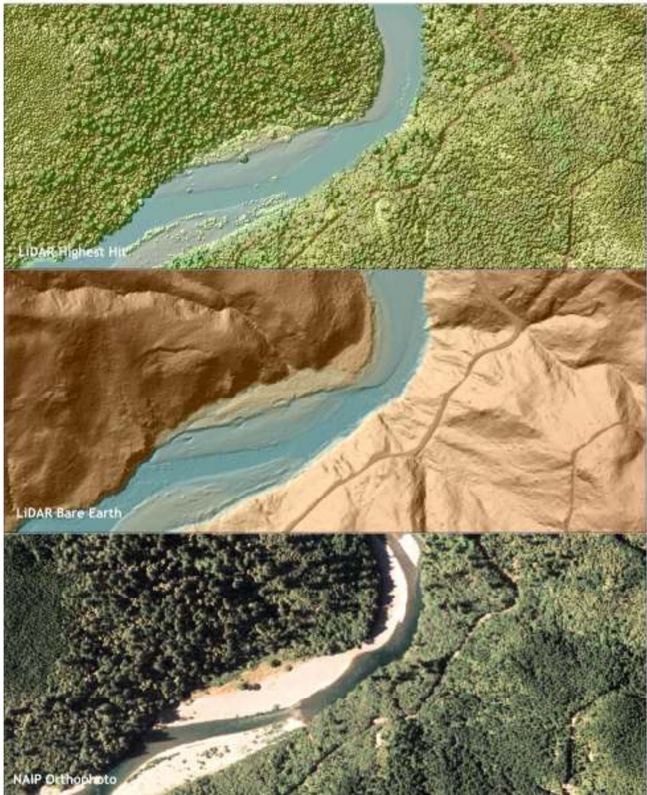
Figure 4.7. Chetco River upstream of confluence with Elk Creek (quad 42124-b2). Upper image derived from highest hit LiDAR, center image derived from bare earth LiDAR, lower image derived from NAIP orthophoto.
