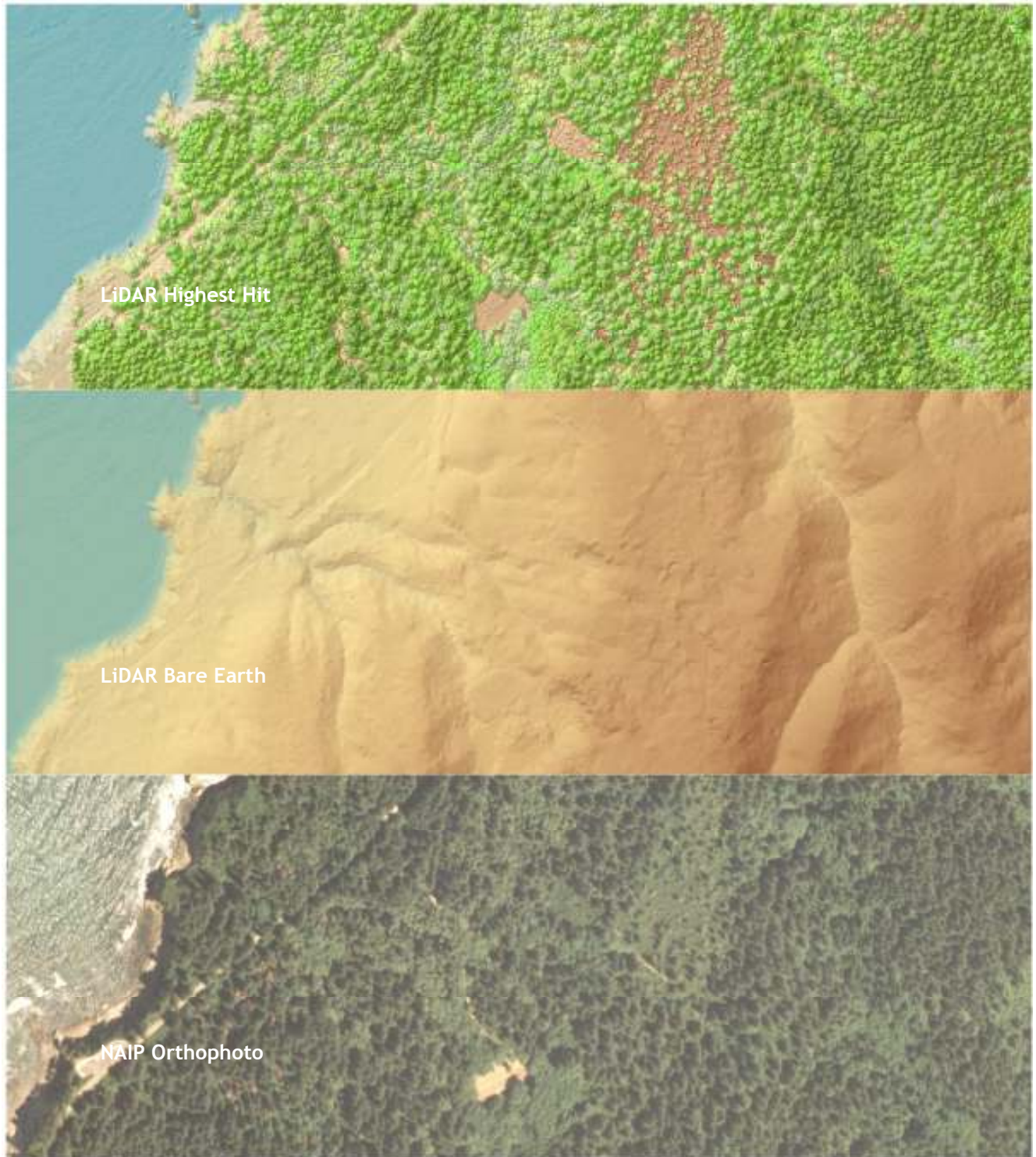
Figure 4.12. Coast beach north of Cape Arago State Park in delivery tile 43124C4. Upper image derived from highest hit LiDAR, center image derived from bare earth LiDAR, lower image derived from NAIP orthophoto.
