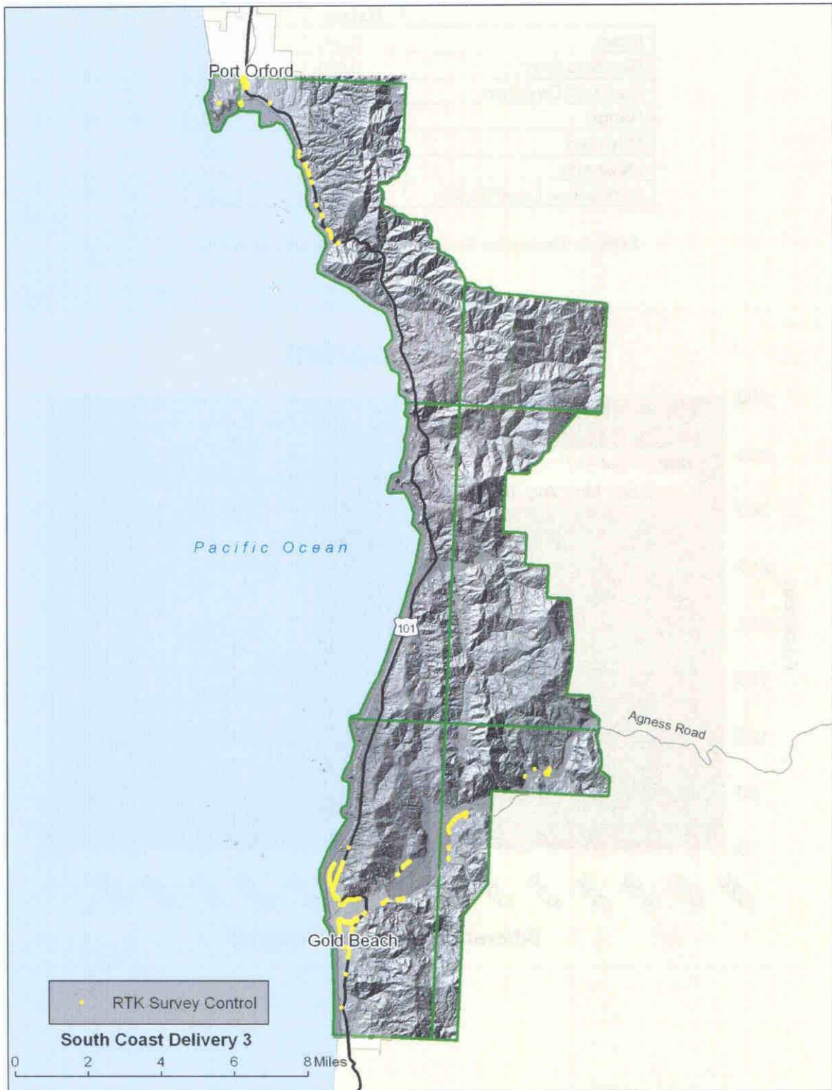
Figure 6. Locations of RTK control surveyed by DOGAMI. Data was used to test absolute accuracy for the South Coast lidar survey within the Delivery 1 extent.
