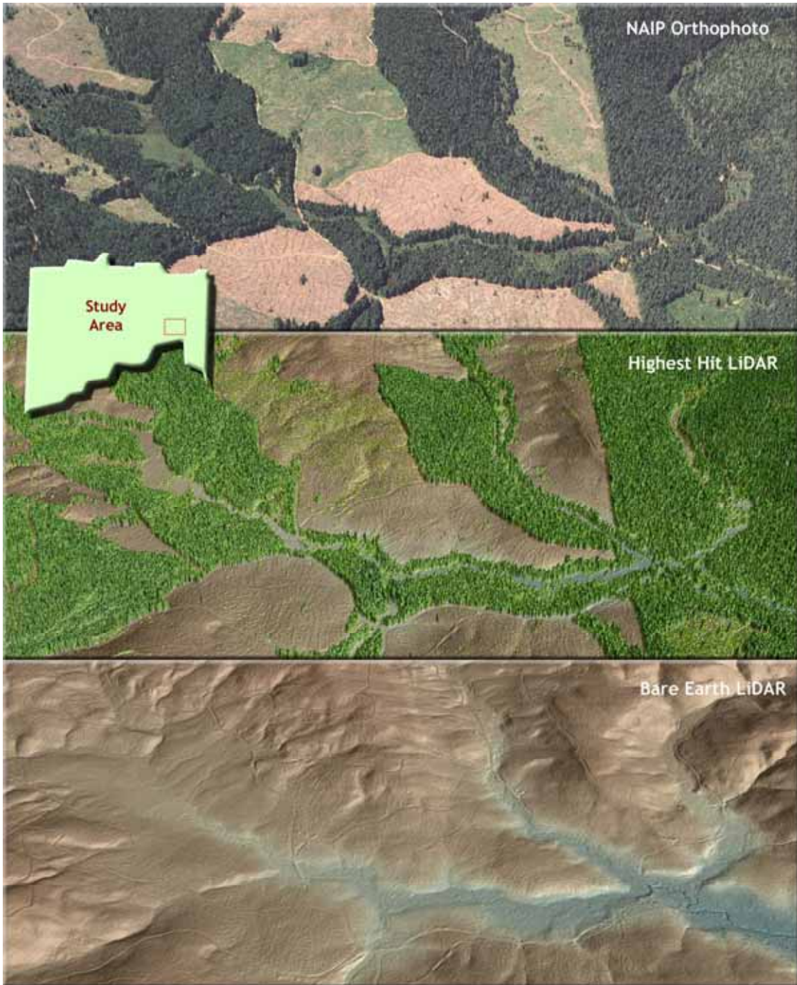
Figure 35. 3-d oblique view of LiDAR-derived surfaces showing a view of the Devils Lake Fork upper watershed.
