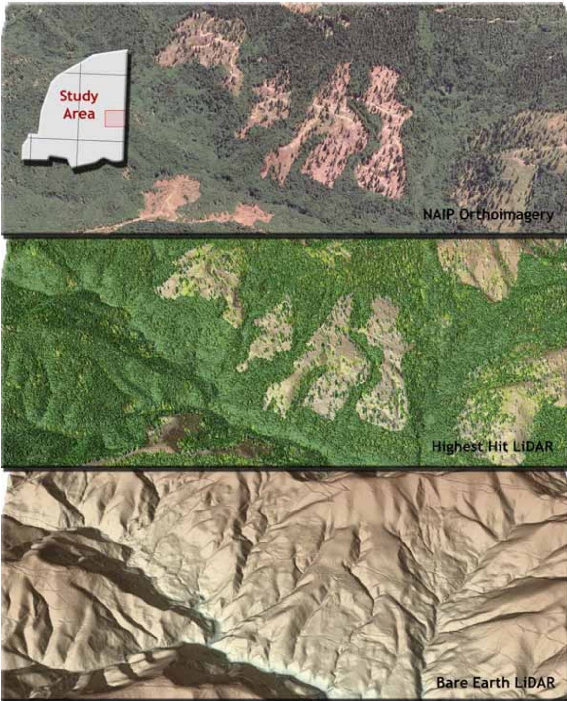
Figure 34. 3-d oblique view of LiDAR-derived surfaces in 7.5' Quad 45123E6, showing the upper portion of the Little North Fork Wilson River watershed in the ODF South study area.
