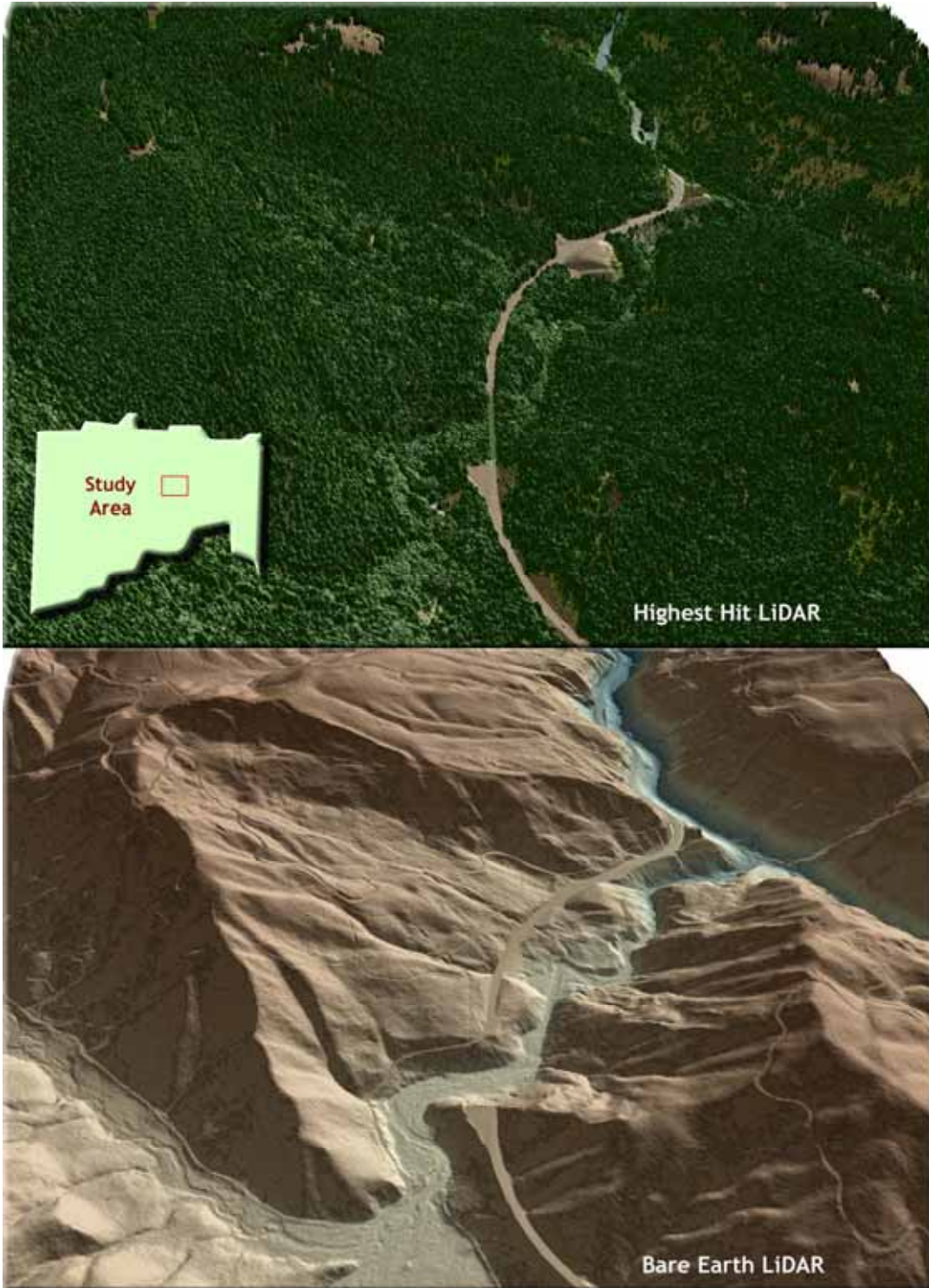
Figure 38. 3-d oblique view of LiDAR-derived surfaces showing an historic landslide along Devils Lake Fork, between Elliot Creek and Drift Creek.
