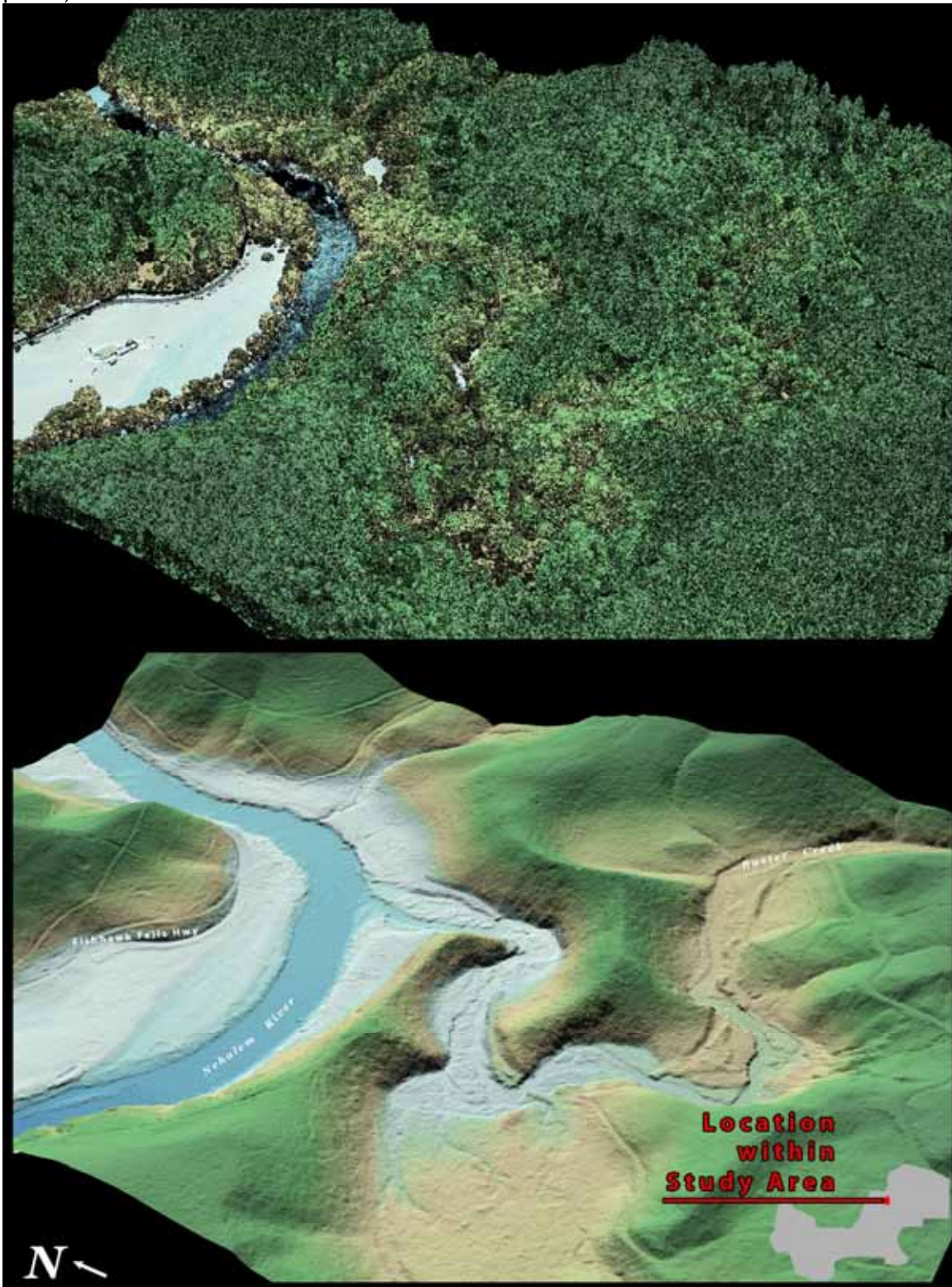
Figure 26. 3-d oblique view of LiDAR-derived surfaces in Quad 45123G6414, showing the confluence of Buster Creek with the Nehalem River, and Fishhawk Falls Road in the ODF North Study Area. (Top image derived from all points, bottom image derived from ground-classified points).
