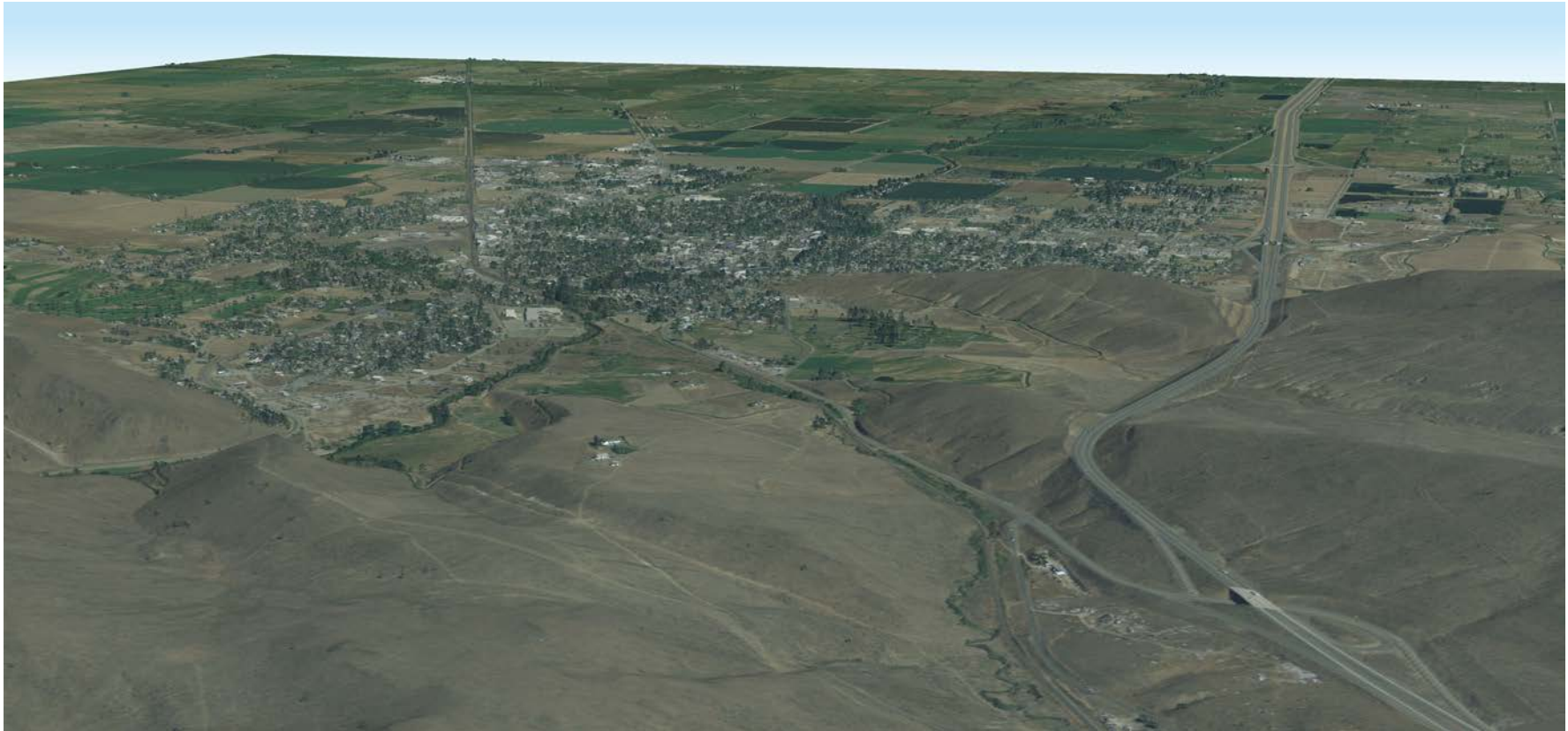
Figure 7.1. Baker City. Image is a three-dimensional LiDAR point cloud with RGB values extracted from a 2010 NAIP orthophoto.
