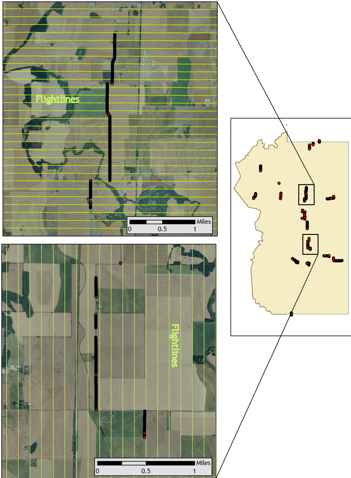
Figure 1.7. RTK point locations in the study area for delivery areas 4 and 5; images are NAIP orthoimages.
