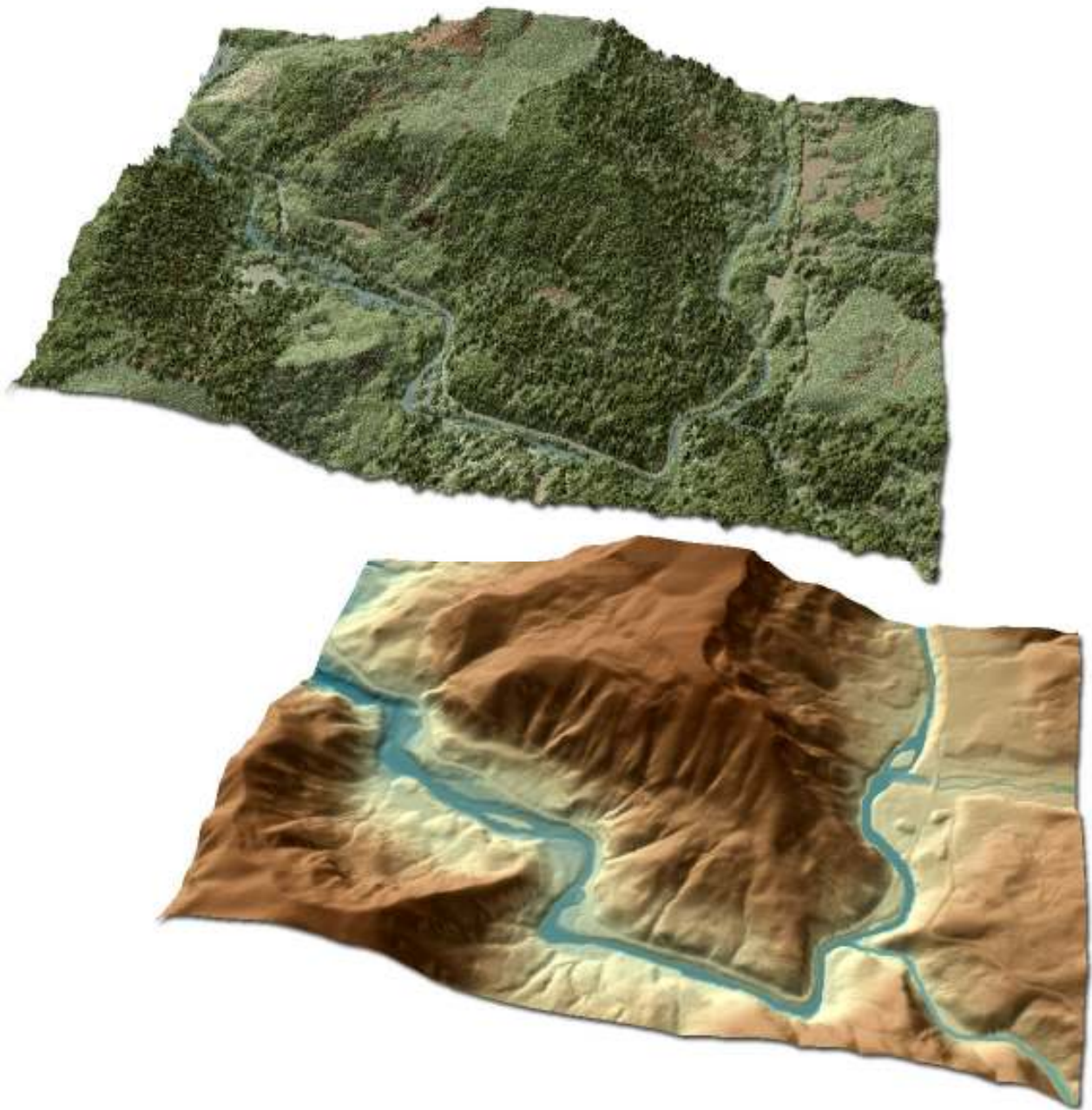
Figure 5.2. Section of Upper Nestucca River in Siuslaw National Forest, viewed from the south. Top image derived from highest hit LiDAR, bottom image derived from bare earth LiDAR.
