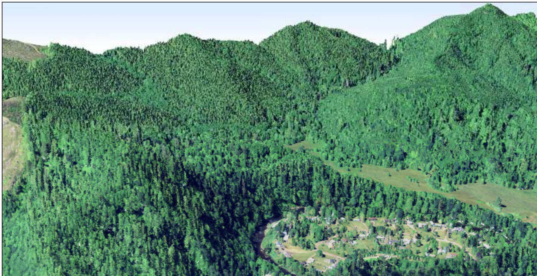
Figure 5.3. Siuslaw National Forest near Blaine Road, East of Beaver, Oregon. Image is a three dimensional LiDAR point cloud with RGB values extracted from a NAIP orthophoto.
