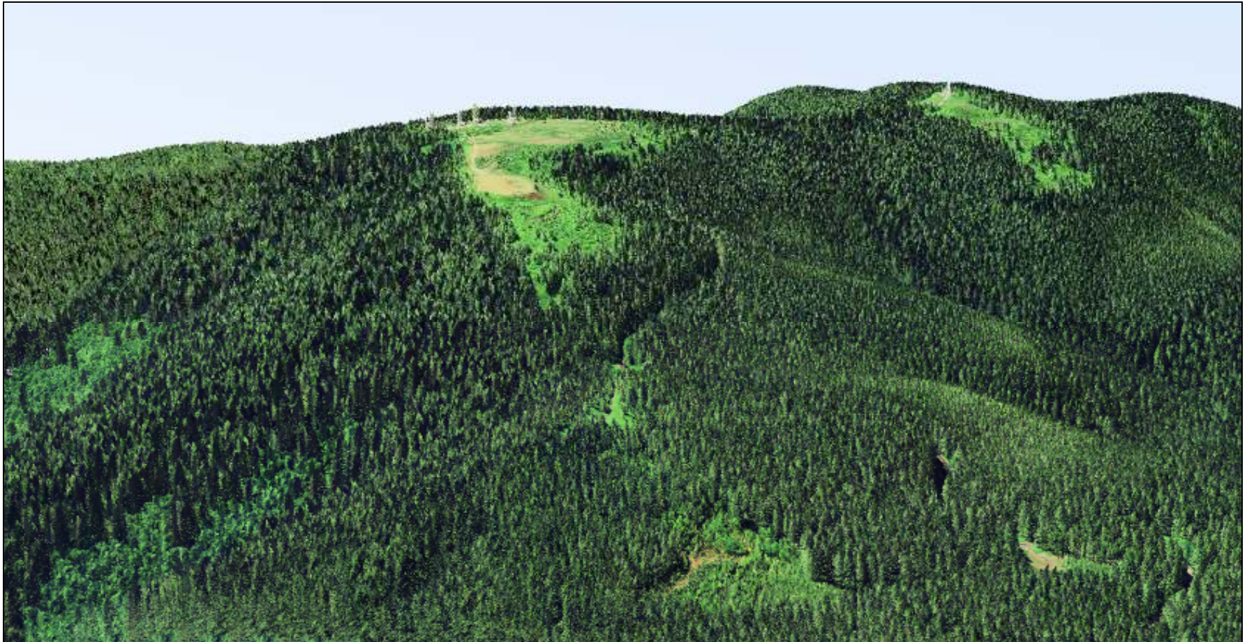
Figure 5.4. Summit of Mount Hebo. Image is a three dimensional LiDAR point cloud with RGB values extracted from a NAIP orthophoto.
