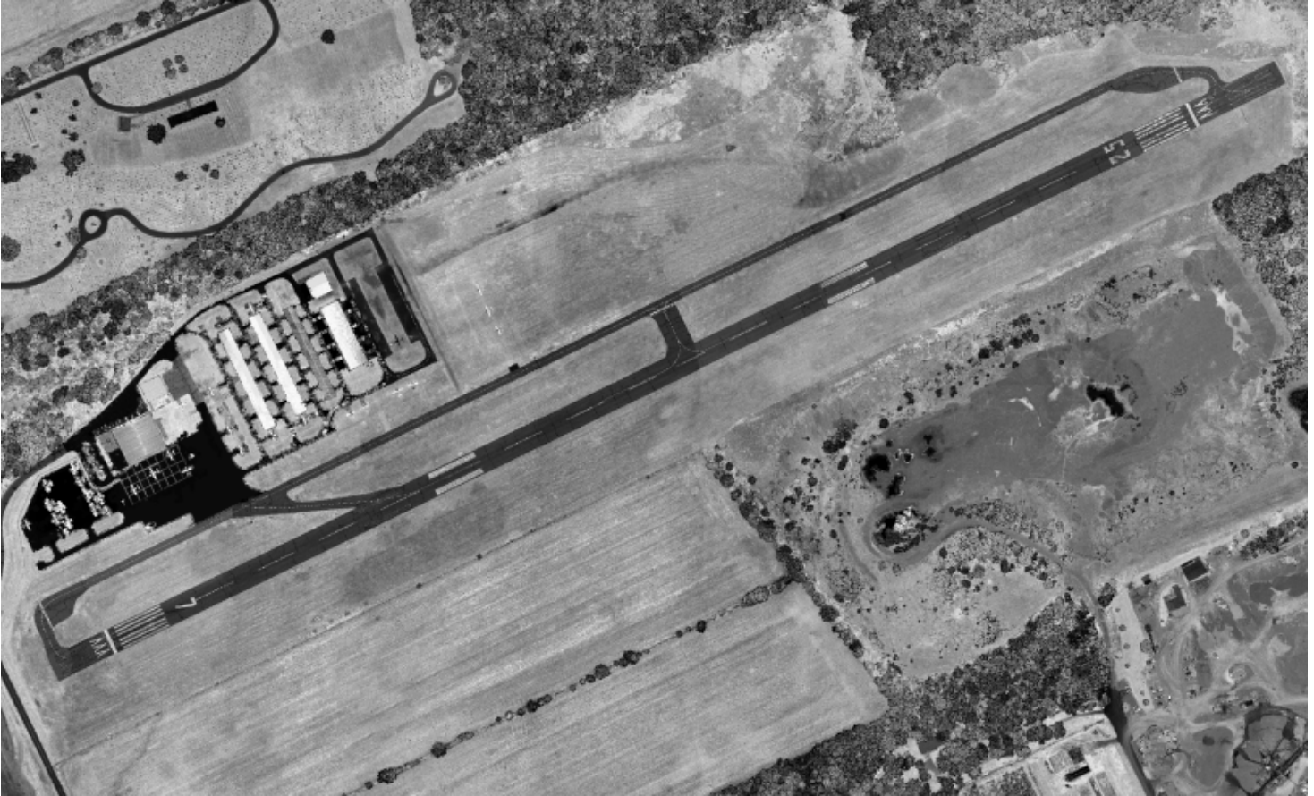
Figure 7-4: Ortho photo generated from LiDAR intensity reflectance.
