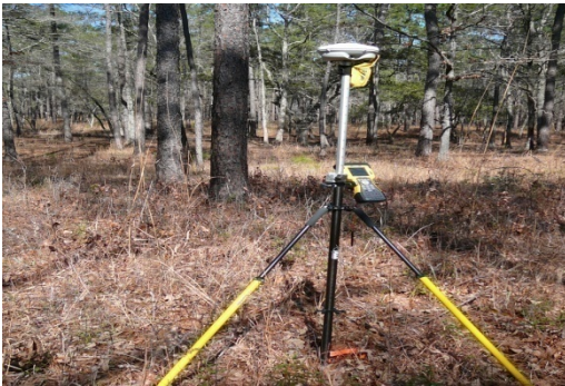
W_8-05-05 – Survey photo- In the forest. Delta Z between LiDAR and GPS is about 10 ft.
