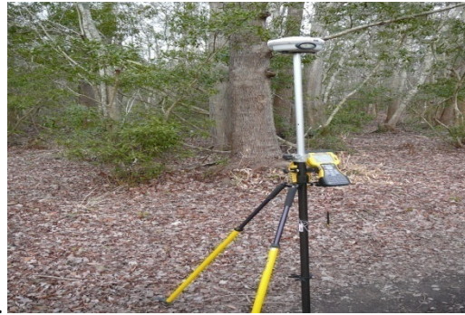
U_8-07-12 – Survey photo-In the forest. Delta Z between LiDAR and GPS is about 20ft.
