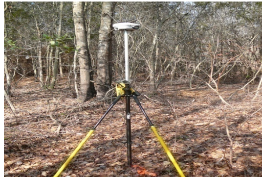
W_8-07-02 – Survey photo- In the forest. Delta Z between LiDAR and GPS is about 6 ft.
