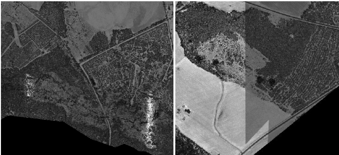
Figure 6 – Left intensity image shows white stripes at nadir. Right image shows tonal changes within a tile.
