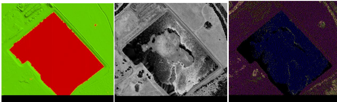
Figure 17 – 4879-04 Misclassification of ground points. Left image is ground density model and middle is full point cloud with intensity. Right image is full point cloud colored by classification, yellow is unclassified (class 1), purple is ground (class 2), and blue is water (class 9). Bottom image is profile of cross-section.
