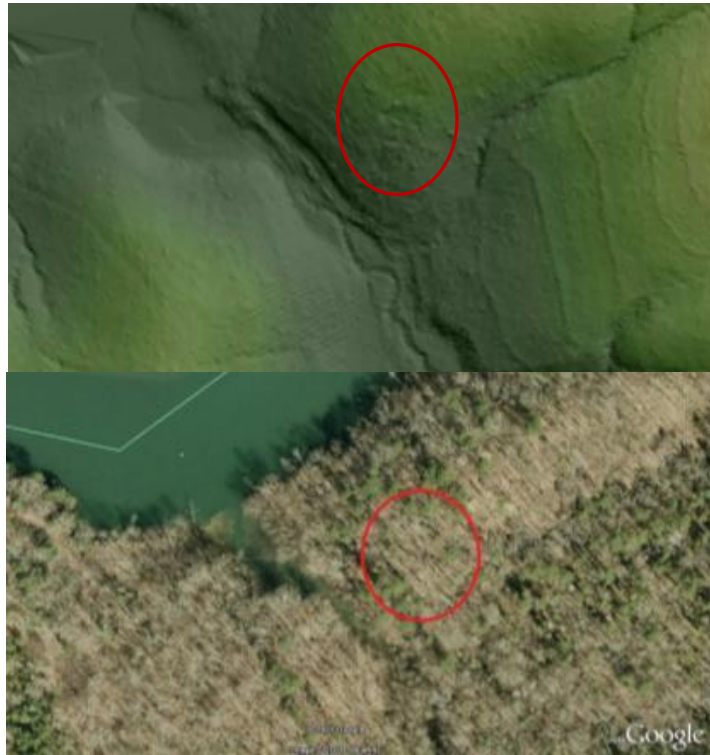
Figure 3 – TIN model of the area before final edits and hydro-flattening have been applied (top) and aerial imagery of the same area.
