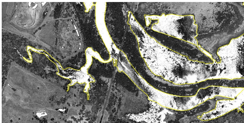
Figure 10 – Hydro breakline check for tile 3197_30_2_a.las. Yellow lines are collected hydro features.
