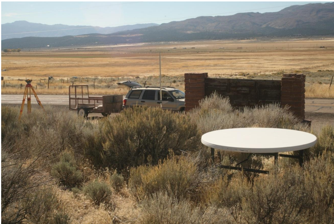
Figure 1. Example of lidar target along with equipment used to level its height relative to a nearby benchmark.
