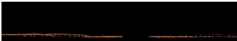
Figure 17 - Same profile as image above, but with all points turned off except for ground points. No extraneous points exist in the ground model.
