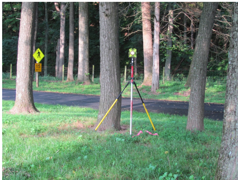
Figure 8: Survey Checkpoint FO-12. This checkpoint is located right next to a large tree. Checkpoints must not be located next to obstructions as this can prevent the LiDAR sensor from reaching its target. Due to the poor placement of this checkpoint, it was not used during vertical accuracy testing.
