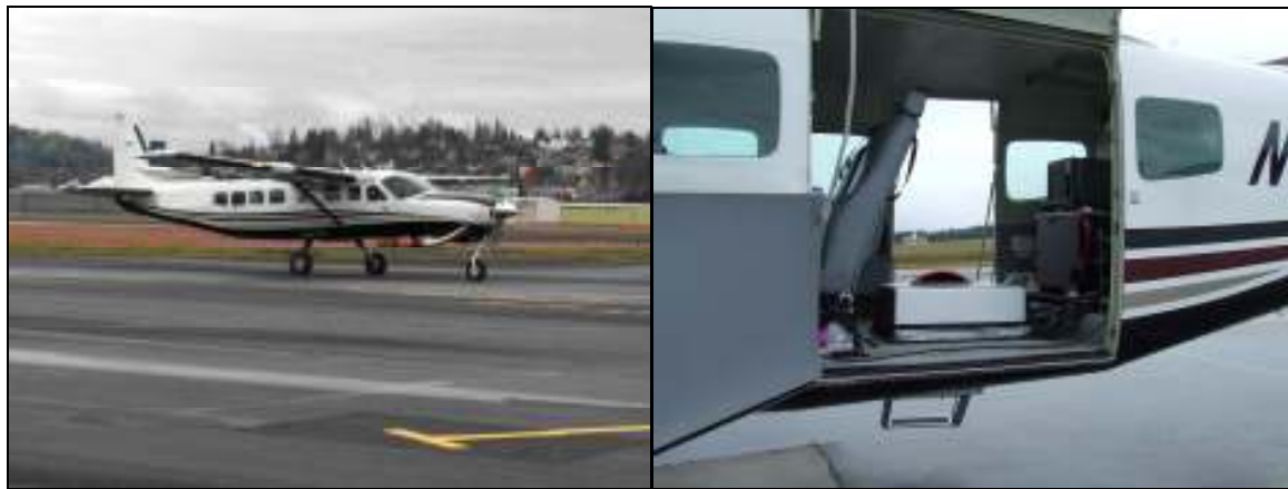
The Cessna Caravan is a powerful, stable platform, which is ideal for the often remote and mountainous terrain found in the Pacific Northwest. The Leica ALS50 sensor head installed in the Caravan is shown on the right.
