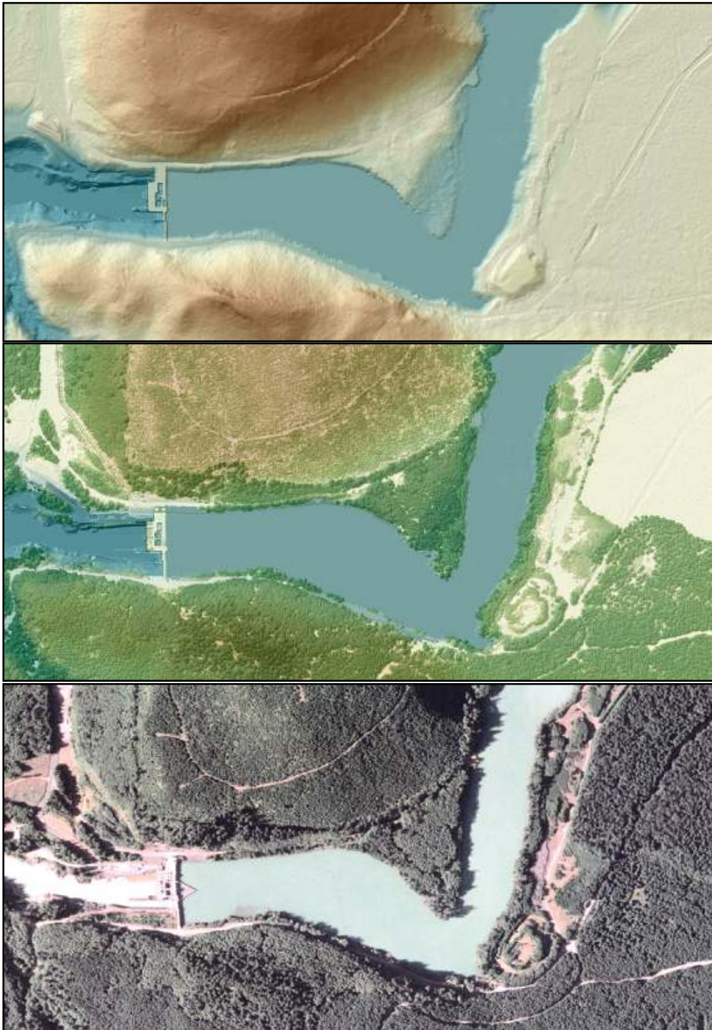
Figure 8.7. Plan view showing the Cowlitz River, the Cowlitz Falls Dam and Lake Scanewa (top image is derived from ground-classified LiDAR points, middle image is derived from highest hit classified LiDAR points and bottom image is an orthophoto).
