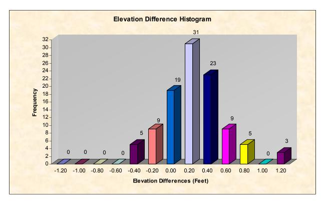
Figure 4 – Histogram of Elevation Discrepancies within 0.2 ft bands
