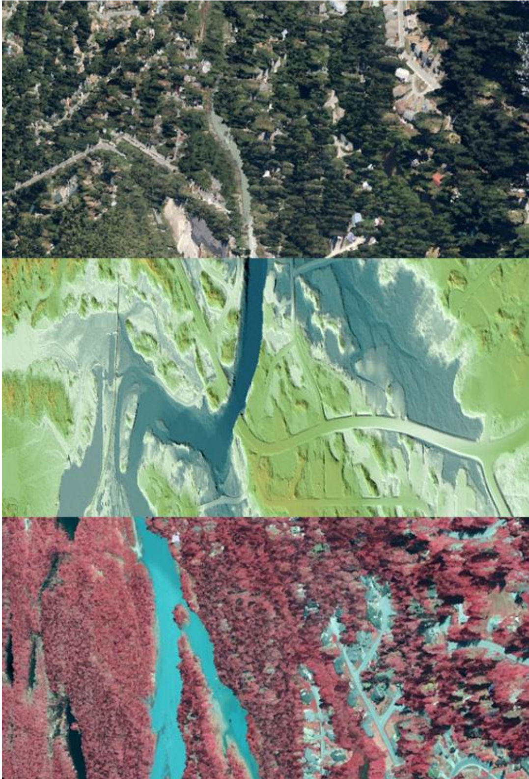
Figure 21: View looking east over Back Loop Juneau near Mendenhall Lake. The image was created from LiDAR point cloud colored by NIR imagery (left), gridded ground-classified LiDAR points colored by elevation (center), and RGB imagery (right).
