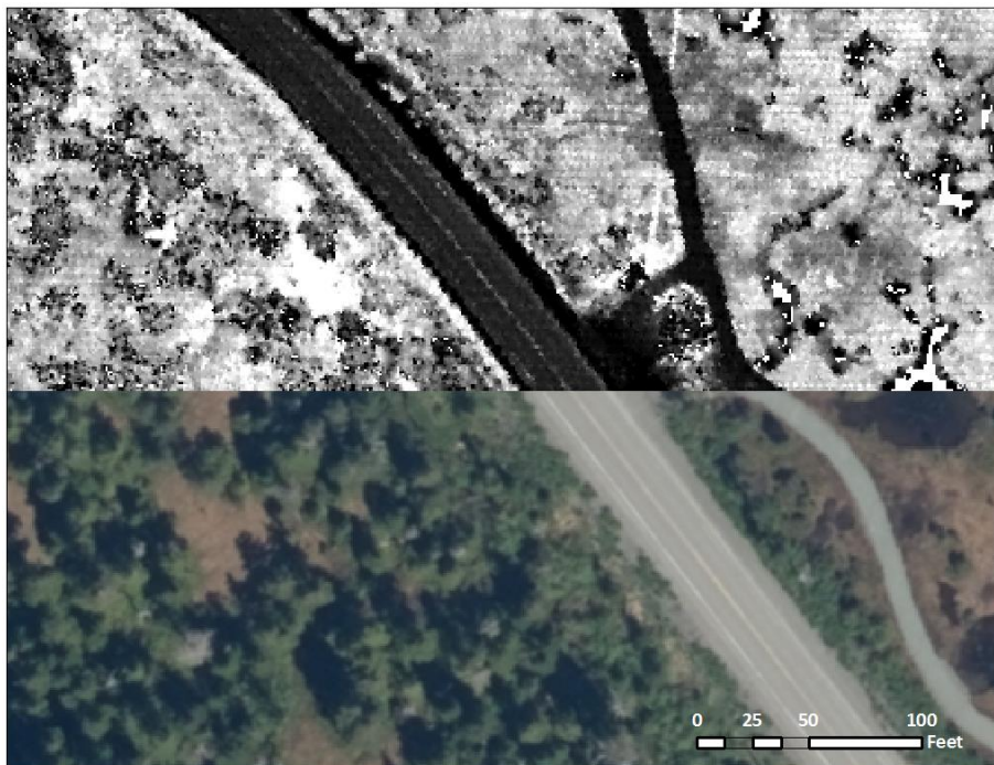
Figure 18: Image displaying the co-registration between the LiDAR intensity image and the 30 cm orthophoto at a location within the Juneau LiDAR and Imagery Priority 1 area.
