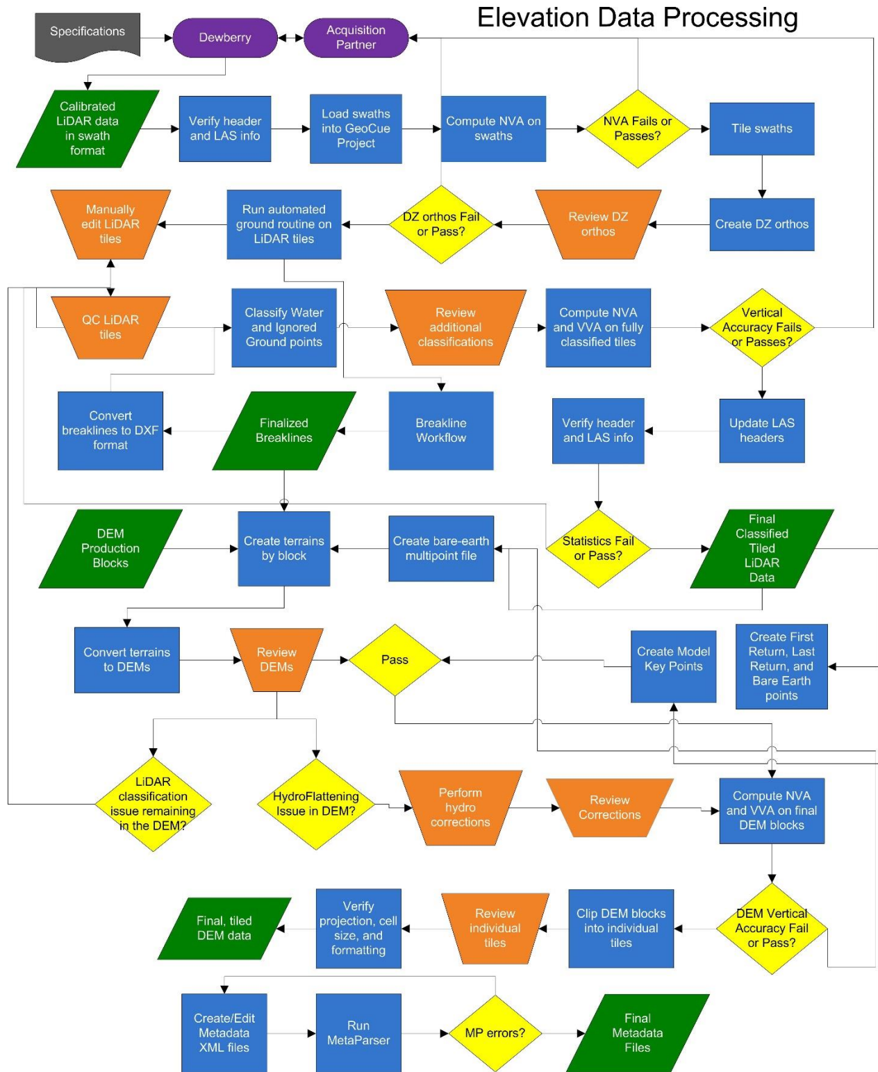
Figure 25-DEM Production Workflow
