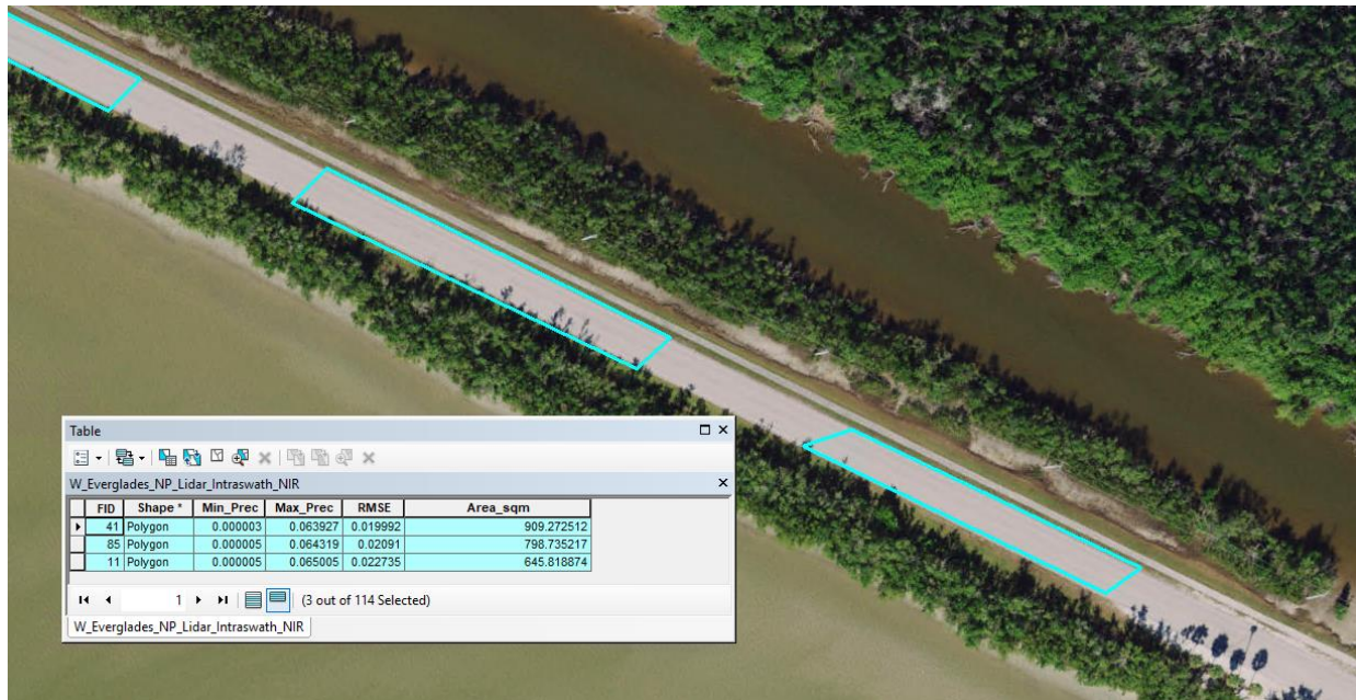
Figure 8. Intraswath polygons used to test intraswath vertical accuracy
