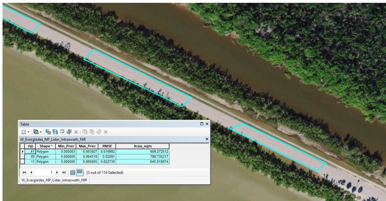
Figure 8. Example test polygon for intraswath testing, and its results
