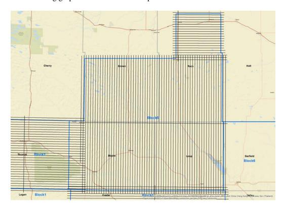
Lidar data was acquired leaf-off, snow-free and while water bodies are at below to normal levels by Surdex from December 23, 2016 to June 2, 2017. Surdex utilized their single engine Cessna 206 with Optech Galaxy-5060382 multi-pulse sensor. Surdex set up GPS base stations for all flights at or near Ainsworth or Rock County Regional Airports. All flight lines were within 40 miles of a GPS station.
