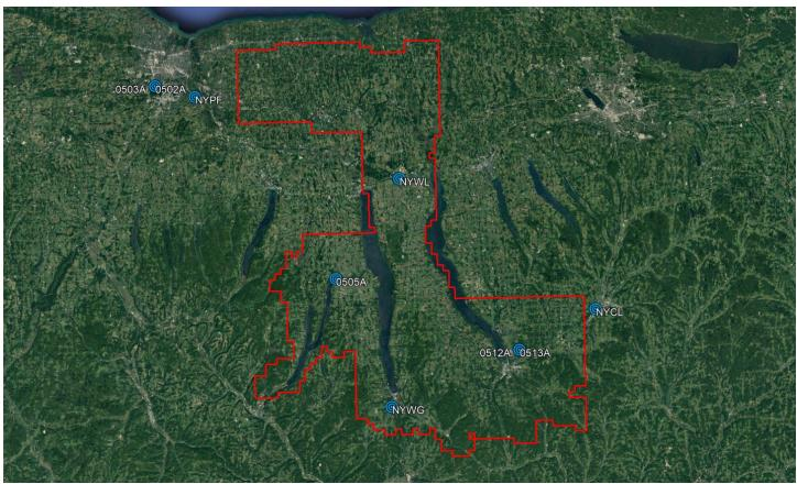
Figure 4: GNSS Reference Stations
