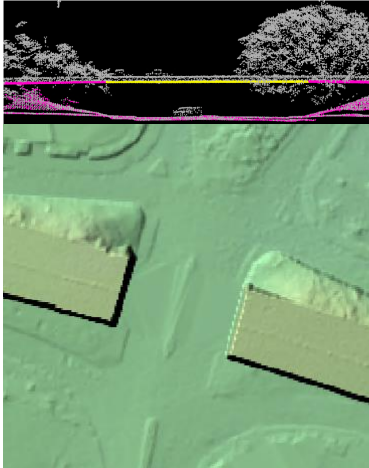
Figure 18 – Tile number 19QHA37506750. The DEM in the bottom view shows an area where a bridge has been removed from ground. The surface model must make a continuous model and in order to do so, points are connected through interpolation. This results in less detail where the surface must be interpolated. The profile in the top view shows the lidar points of this particular feature colored by class. All bridge points have been removed from ground (pink) and are bridge decks (yellow).
