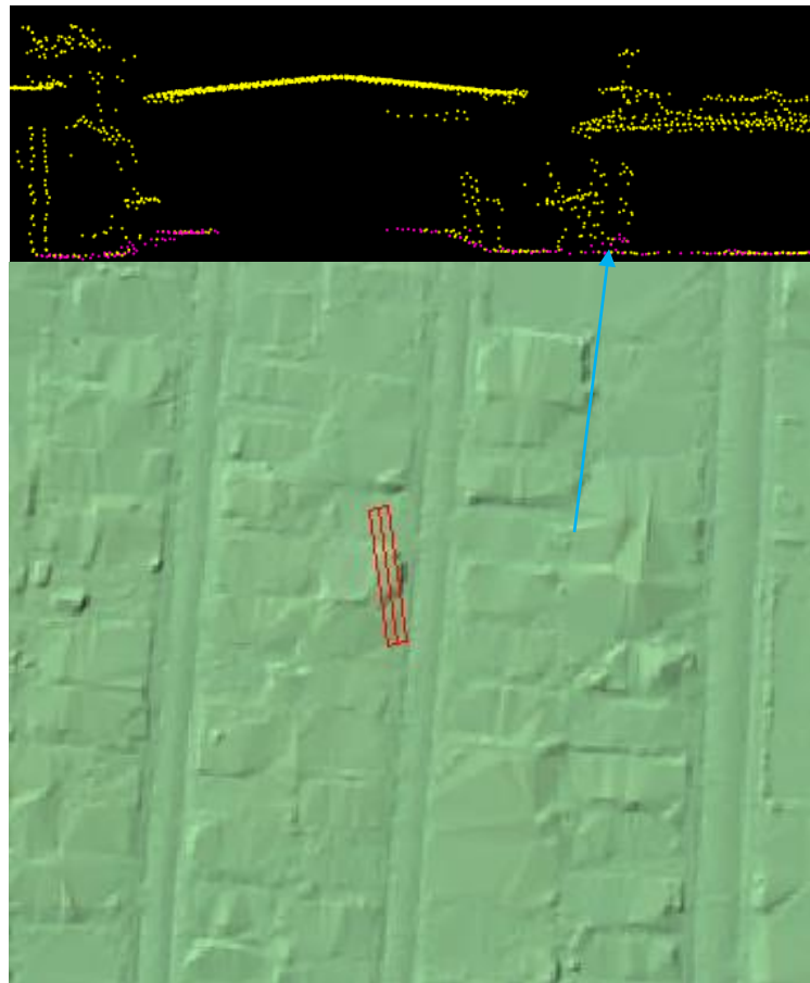
Figure 17 – Tile number 19QHA39006750. Profile with points colored by class (class 1=yellow, class 2=pink) is shown in the top view and a TIN of the surface is shown in the bottom view. The arrow identifies low vegetation points. A limited number of these small features are still classified as ground but do not impact the usability of the dataset.
