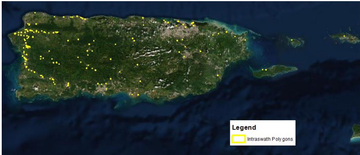
Figure 11 - Intraswath polygons used to test intraswath vertical accuracy.
