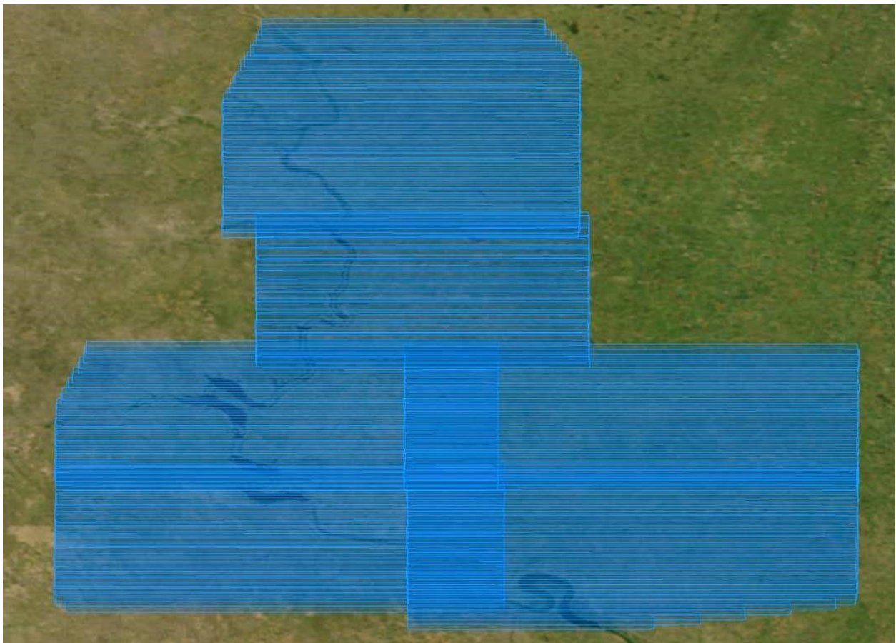
Figure 3 – Lidar swath output showing complete coverage.
