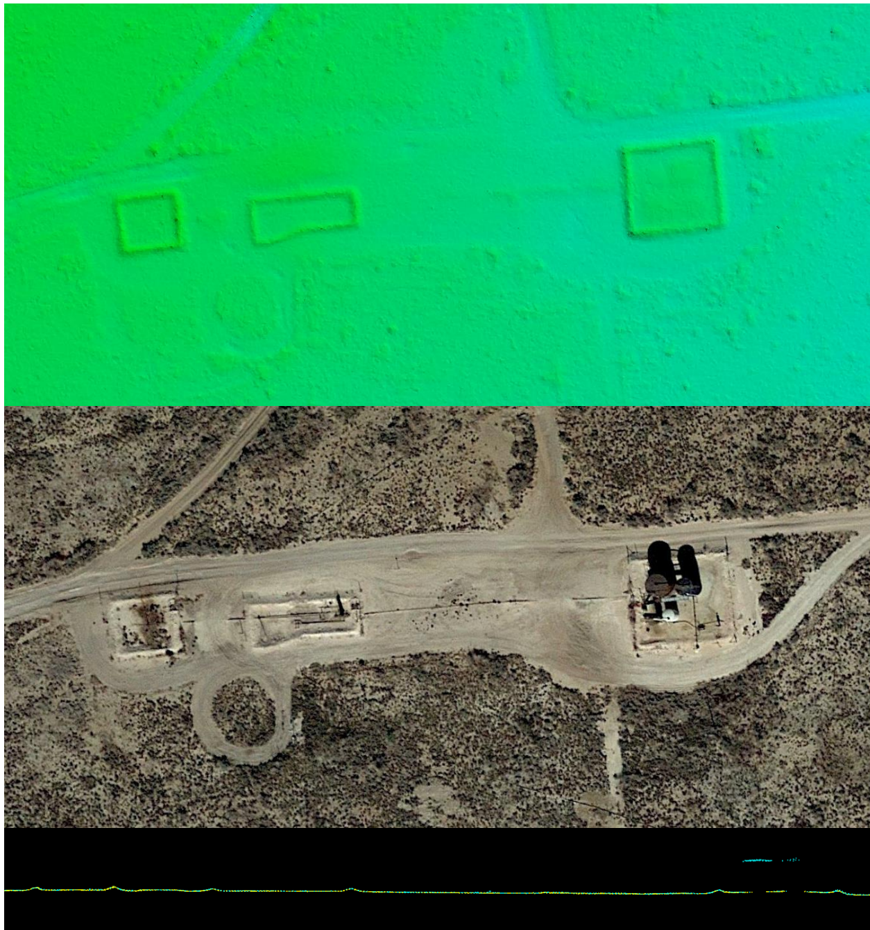
Figure 93 – Tile 13SGR110445. The top view is a tin surface that shows the berms created, the image in the middle shows the working structures in the area and a profile with the points colored by class (class 1=cyan, class 2=yellow) is shown in the bottom view.
