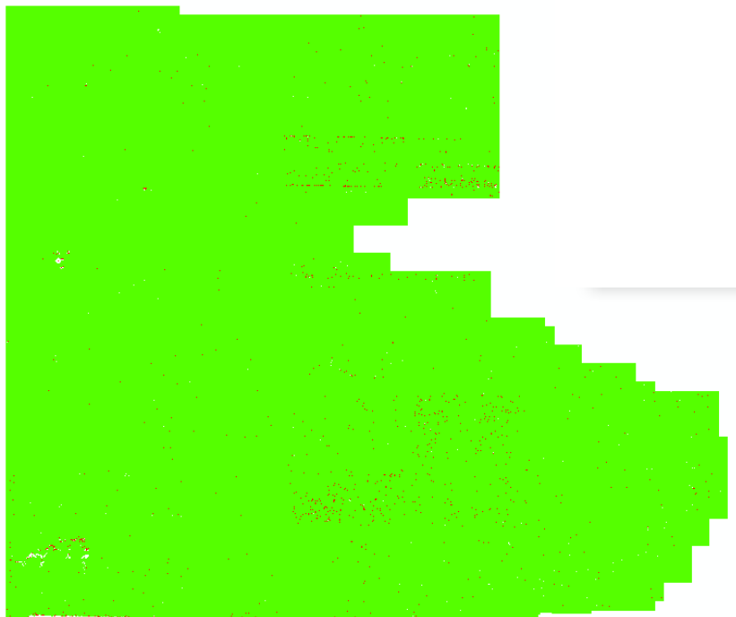
Figure 66– 1-square meter density grid for Block 12. There are some 1-meter cells that do not contain 2 points per square meter (red areas) due to the irregular spacing of lidar point cloud data. Most 1-square meter cells contain at least 2 points per square meter (green areas) showing there are no systematic density issues. When density is viewed/analyzed by representative 1-square kilometer areas, density passes with no issues.
