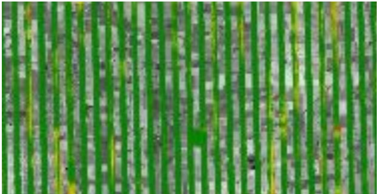
Figure 27 – QC block colored by distance to ensure accuracy at swath edges.
