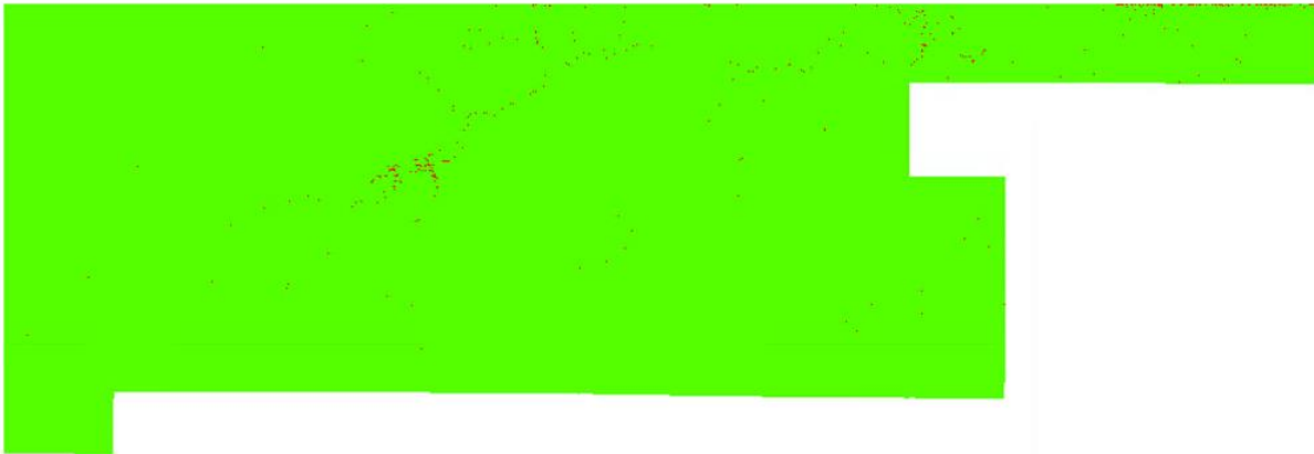
Figure 77– Spatial Distribution for Block 09. All cells (2*NPS cellsize) containing at least one lidar point are colored green. Cells that do not contain a lidar point, including water bodies which are acceptable NoData area, are colored red. Without removing acceptable NoData areas due to water, at least 98% of cells contain at least one lidar point.
