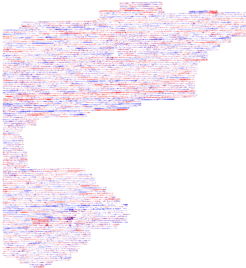
Figure 38 – QC block colored by distance to ensure accuracy at swath edges.
