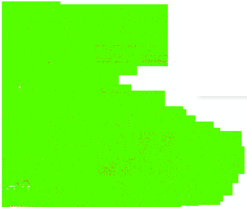
Figure 66– 1-square meter density grid for Block 12. There are some 1-meter cells that do not contain 2 points per square meter (red areas) due to the irregular spacing of lidar point cloud data. Most 1-sqaure meter cells contain at least 2 points per square meter (green areas) showing there are no systematic density issues. When density is viewed/analyzed by representative 1-square kilometer areas, density passes with no issues.
