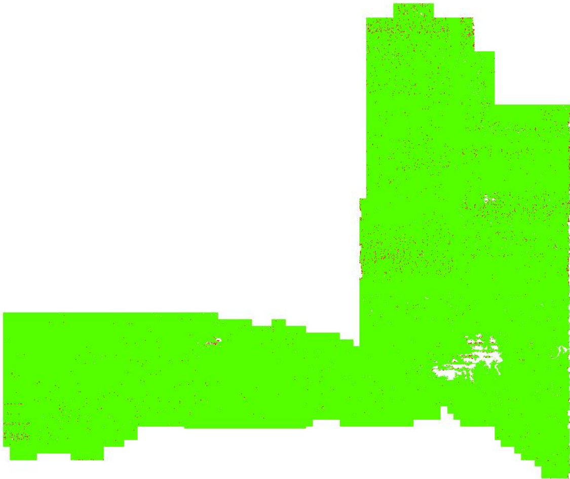
Figure 67– 1-square meter density grid for Block 13. There are some 1-meter cells that do not contain 2 points per square meter (red areas) due to the irregular spacing of lidar point cloud data. Most 1-square meter cells contain at least 2 points per square meter (green areas) showing there are no systematic density issues. When density is viewed/analyzed by representative 1-square kilometer areas, density passes with no issues.
