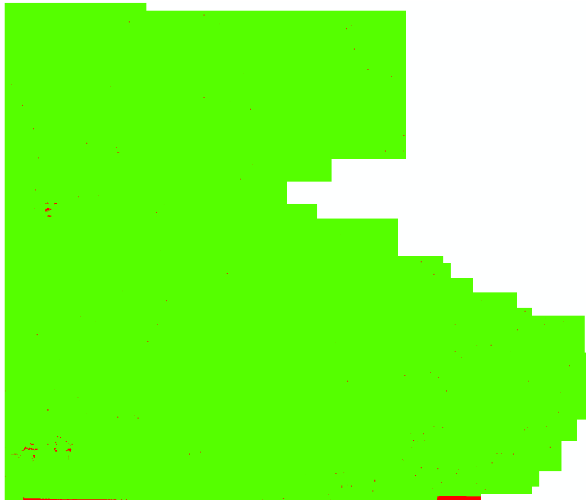
Figure 80– Spatial Distribution for Block 12. All cells (2*NPS cellsize) containing at least one lidar point are colored green. Cells that do not contain a lidar point, including water bodies which are acceptable NoData area, are colored red. Without removing acceptable NoData areas due to water, at least 98% of cells contain at least one lidar point.
