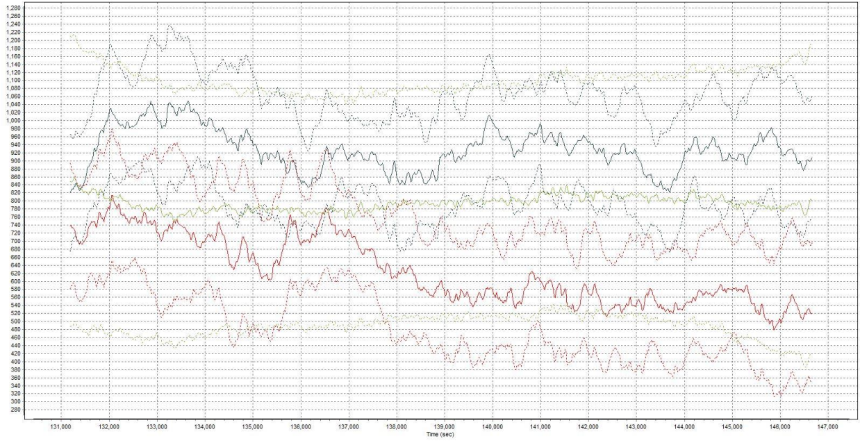
— x accelerometer bias (micro-g) — y accelerometer bias (micro-g) — z accelerometer bias (micro-g)
