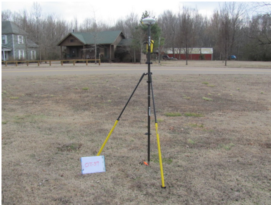
Figure 29-Field Photo for checkpoint OT-39. Field photo shows the checkpoint should be located within short grass, but final coordinates locate checkpoint in an asphalt driveway. Review by the surveyor deemed this survey checkpoint erroneous and unsuitable to use in the final vertical accuracy testing.
