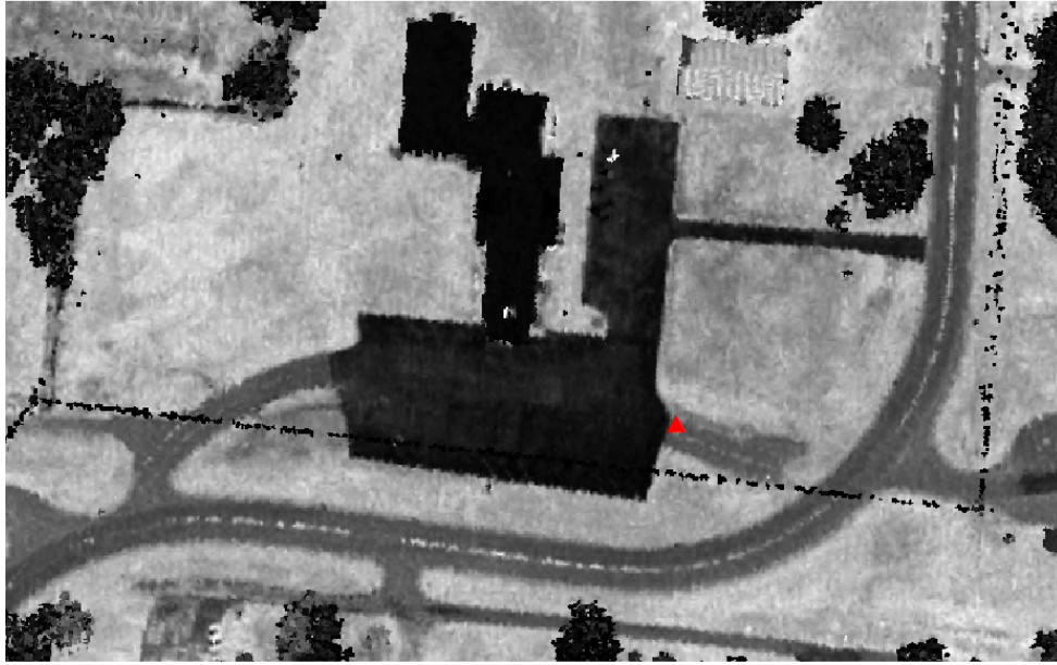
Figure 30-Tile 16SCE5240. Intensity imagery is shown with checkpoint OT-39 (red triangle) overlaid. Field sketch and field photo show the checkpoint should be located within short grass, but final coordinates locate checkpoint in an asphalt driveway. Review by the surveyor deemed this survey checkpoint erroneous and unsuitable to use in the final vertical accuracy testing.
